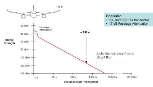
Figure 2: RF power level from an RLAN on board aircraft
