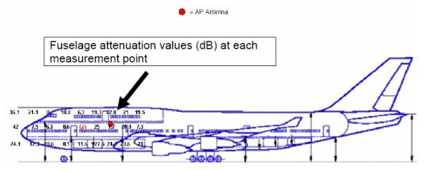
Figure 1: Measurement of fuselage Attenuation
