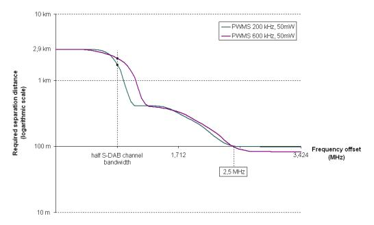
Figure 12: Separation distance required from an indoor adjacent channel PWMS interferer (50 mW, 200 kHz and 600 kHz, single carrier interference) for wall absorption = 10dB
