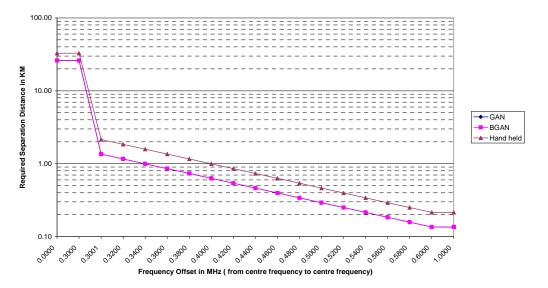
Figure 16: Required separation distance from PWMS interferer (50 mW and 600 kHz; building attenuation = 10 dB) under "free space attenuation up to 5 km and 40 log d attenuation beyond 5 km" propagation model
