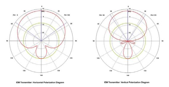
Figure 5: PWMS IEM Antenna Pattern above 1525 MHz
