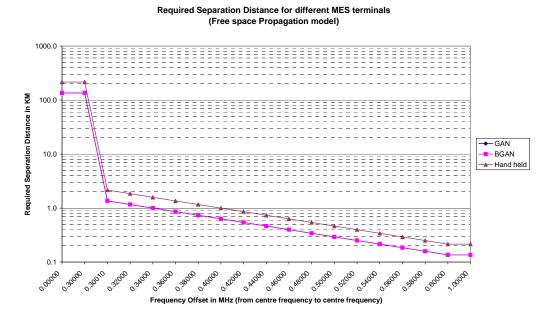
Figure 15: Required separation distance from PWMS interferer (50 mW and 600 kHz; building attenuation = 10 dB) under free space propagation model
