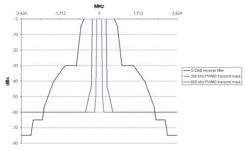
Figure 10: S-DAB and PWMS spectrum masks
