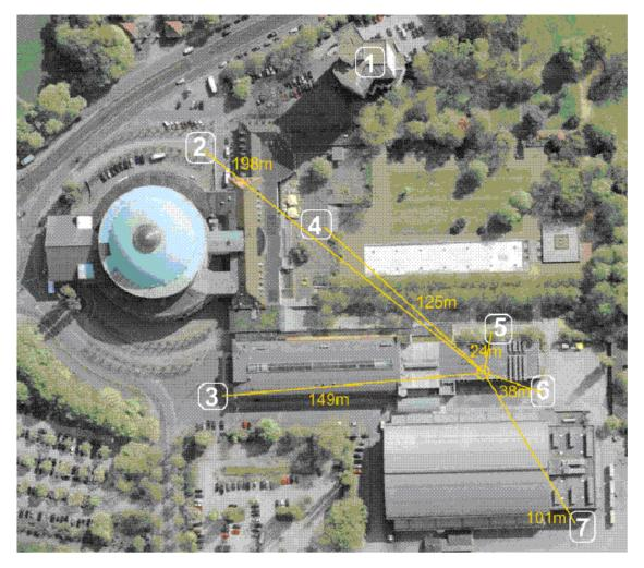
Estimation of additional path loss due to surrounding buildings Path calculated from Kuppelsaal to outdoor test points @1500 MHz
