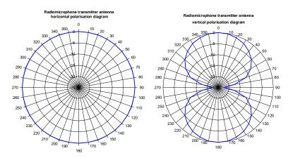
Figure 3: PWMS Body Worn Antenna Pattern below 1525 MHz
