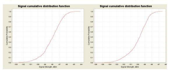
Figure 33: CDF graphs for the ac-MS for 900 MHz at 8000 m (left) and 10000 m (right) above ground
