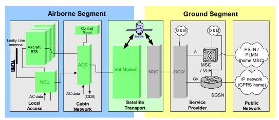
Figure 2: Overall end-to-end architecture of a complete GSMOB system
