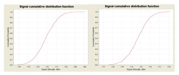
Figure 35: CDF graphs for the ac-MS for 1800 MHz at 8000 m (left) and 10000 m (right) above ground
