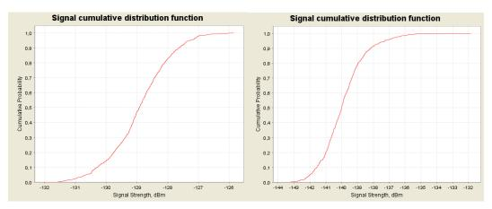
Figure 66: CDF graphs for the ac-MS for 1800 MHz at 3000 m (left) and 5000 m (right) above ground
