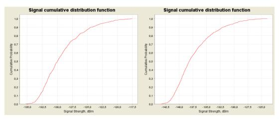
Figure 50: CDF graphs for the NCU (UMTS) for 1800 MHz at 3000 m (left) and 5000 m (right) above ground
