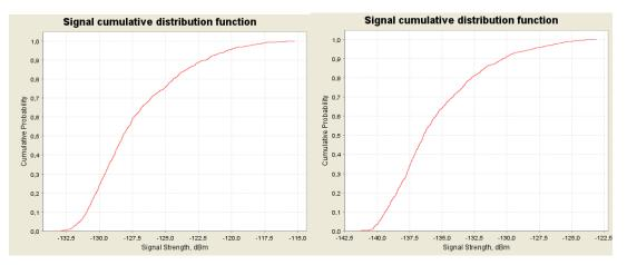
Figure 46: CDF graphs for the NCU (GSM) for 1800 MHz at 3000 m (left) and 5000 m (right) above ground
