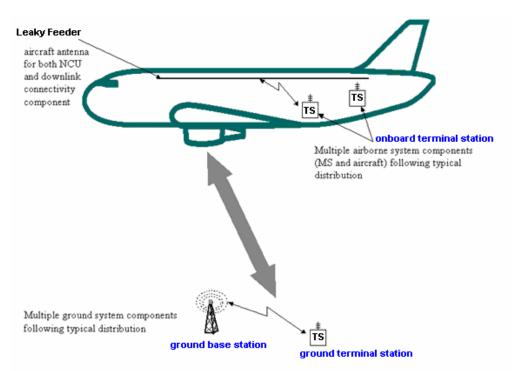
Figure 4: GSMOB and terrestrial cellular system interference scenario
