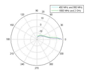
Figure 105: Elevation patterns used for the SEAMCAT simulations
