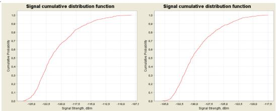
The following figures provide the CDF graphs for the NCU (UMTS) for 900 MHz at 3000, 5000, 8000 and 10000 m above ground.
