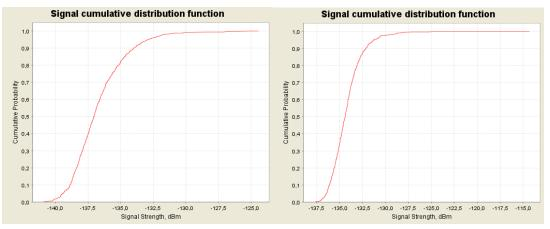
Figure 63: CDF graphs for the multiple ac-BTS for 1800 MHz for normal busy (left) and extreme busy (right) cases for 10 GSM 1800 channels onboard
