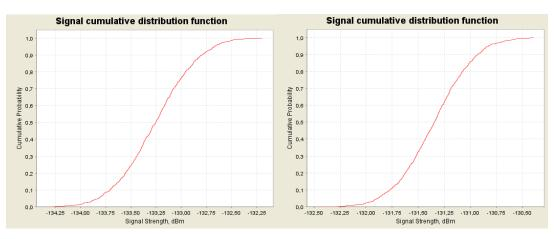
Figure 72: CDF graphs for the multiple ac-MS for 1800 MHz for normal busy (left) and extreme busy (right) cases for 10 GSM 1800 channels onboard
