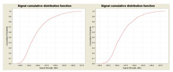
Figure 38: CDF graphs for the NCU (GSM) for 1800 MHz at 3000 m (left) and 5000 m (right) above ground
