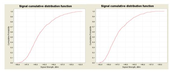
Figure 43: CDF graphs for the ac-BTS for 1800 MHz at 8000 m (left) and 10000 m (right) above ground
