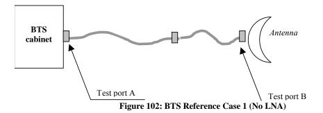
Reference case 1 reflects the configuration assumed for the values referred to in the 3GPP specifications. It consists of a BTS cabinet and antenna where only cable loss and connector loss are considered.
