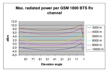
Figure 13: Maximum radiated power in GSM1800 BTS receive channel from different heights
