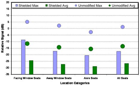
Figure 111: Summary of received signals normalized to theoretical values
