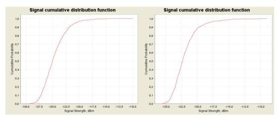
Figure 59: CDF graphs for the multiple NCU (GSM) for 1800 MHz for normal busy (left) and extreme busy (right) cases
