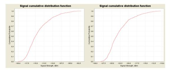
Figure 52: CDF graphs for the NCU (CDMA) for 450 MHz at 3000 m (left) and 5000 m (right) above ground
