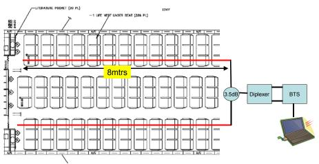
Figure 85: System test setup
