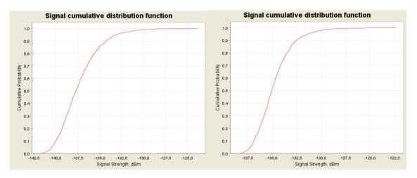
Figure 57: CDF graphs for the multiple NCU (GSM) for 1800 MHz for normal busy (left) and extreme busy (right) cases
