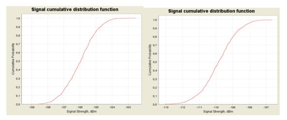
Figure 34: CDF graphs for the ac-MS for 1800 MHz at 3000 m (left) and 5000 m (right) above ground
