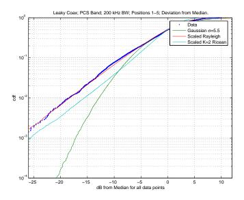
Figure 91: Cumulative distribution of power variation about the median. Leaky feeder antenna, 200 kHz channel bandwidth
