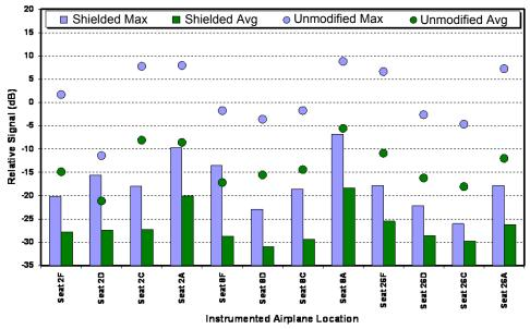
Figure 110: Statistical comparison of received signals normalized to theoretical values
