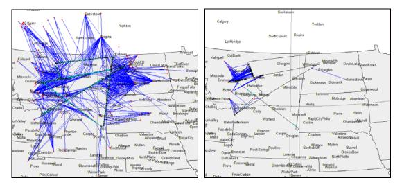
Figure 112: Maps of terrestrial system acquisition during flight. Left: Unmodified aircraft; Right: RF shielded aircraft
