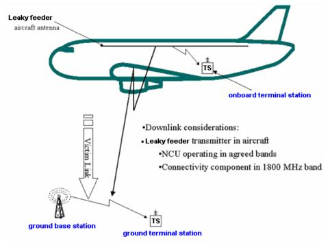
Figure 8: Scenario 3: GSMOB interfering terrestrial victim Downlink (g-BTS/NodeB to g-MS/UE) from a single aircraft
