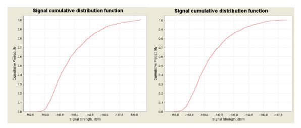
Figure 41: CDF graphs for the NCU (UMTS) for 2000 MHz at 8000 m (left) and 10000 m (right) above ground
