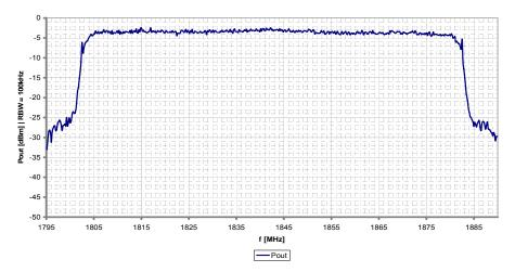
Figure 96: GSM 1800 output spectrum narrow band
