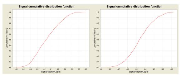
Figure 32: CDF graphs for the ac-MS for 900 MHz at 3000 m (left) and 5000 m (right) above ground
