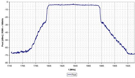
Figure 97: GSM 1800 output spectrum
