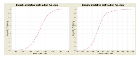
Figure 68: CDF graphs for the ac-MS for 1800 MHz at 3000 m (left) and 5000 m (right) above ground
