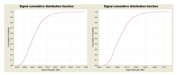
Figure 54: CDF graphs for the multiple ac-BTS for 1800 MHz for 10 GSM 1800 channels onboard for the normal busy (left) and the extreme busy (right) cases
