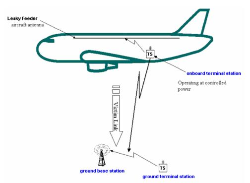
Figure 10: Scenario 5: GSMOB interfering terrestrial uplink (g-MS/UE to g-BTS/NodeB) from a single aircraft
