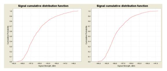
Figure 39: CDF graphs for the NCU (GSM) for 1800 MHz at 8000 m (left) and 10000 m (right) above ground
