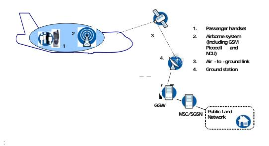
Figure 1: Overview of the GSMOB system and associated terrestrial components
