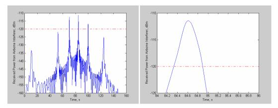
Figure 83: Time history of interference power received by g-MS. 100% coherent array model. Dotted line denotes the (I/N = -6 dB) interference threshold for a GSM mobile. Plot on right is close-up view of the main gain peak
