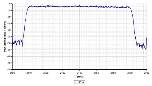
Figure 99: UMTS output spectrum narrow band
