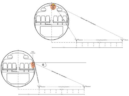
Figure 89: Principle setup aircraft attenuation test
