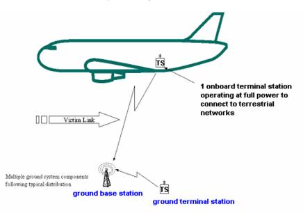
Figure 7: Scenario 2 where ac-MS/UE signal is received by g-BTS/NodeB (no NCU)
