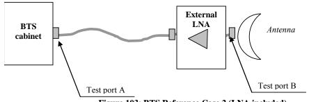
Figure 103: BTS Reference Case 2 (LNA included)
