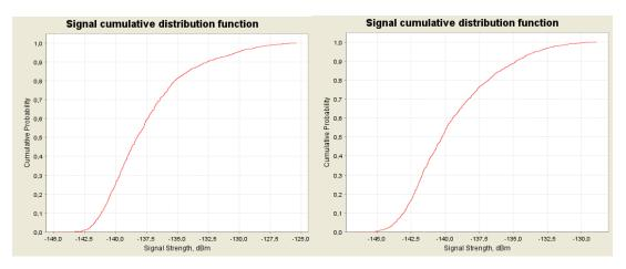
Figure 49: CDF graphs for the NCU (UMTS) for 900 MHz at 8000 m (left) and 10 000 m (right) above ground
