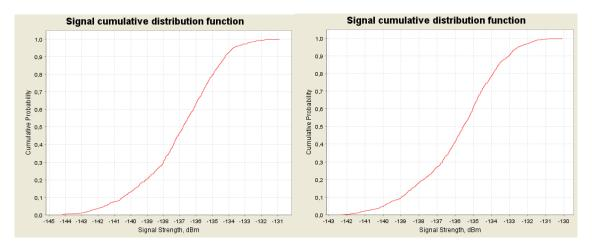
Figure 71: CDF graphs for the multiple ac-MS for 1800 MHz for 50 GSM 1800 channels onboard for the normal busy day (left) and the extreme busy day (right) cases
