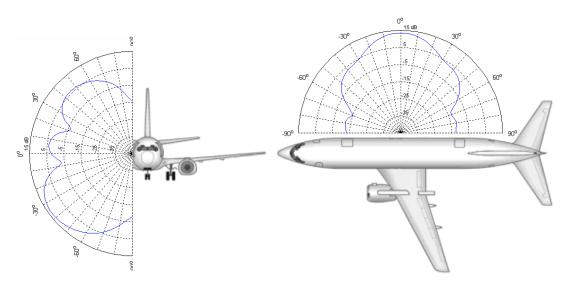
Figure 77: Elevation and azimuth patterns for a single aircraft window coherently illuminated by an isotropic source
