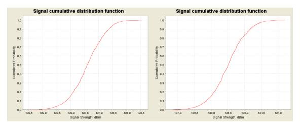
Figure 73: CDF graphs for the multiple ac-MS for 1800 MHz for normal busy (left) and extreme busy (right) cases for 50 GSM 1800 channels onboard
