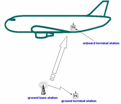
Figure 6: Scenario 1 where g-BTS signal is received by onboard mobile terminals
