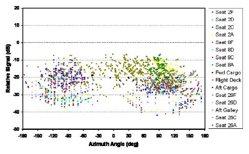
Figure 109: RF Shielded aircraft received signals normalized to theoretical values
