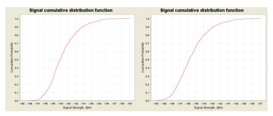
Figure 67: CDF graphs for the ac-MS for 1800 MHz at 8000 m (left) and 10000 m (right) above ground
