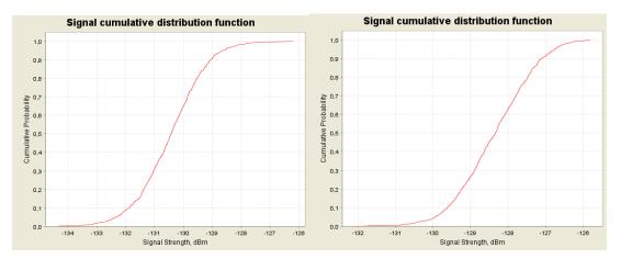
Figure 70: CDF graphs for the multiple ac-MS for 1800 MHz for 10 GSM 1800 channels onboard for the normal busy day (left) and the extreme busy day (right) cases
