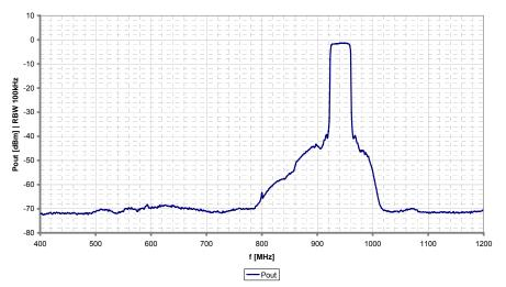
Figure 95: GSM 900 output spectrum wideband
