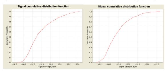
Figure 45: CDF graphs for the NCU (GSM) for 900 MHz at 8000 m (left) and 10000 m (right) above ground
