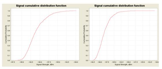
Figure 64: CDF graphs for the multiple ac-BTS for 1800 MHz for normal busy (left) and extreme busy (right) cases for 50 GSM 1800 channels onboard
