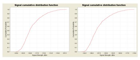
Figure 44: CDF graphs for the NCU (GSM) for 900 MHz at 3000 m (left) and 5000 m (right) above ground
