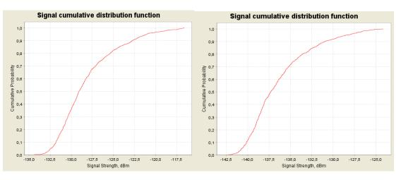
Figure 42: CDF graphs for the ac-BTS for 1800 MHz at 3000 m (left) and 5000 m (right) above ground
