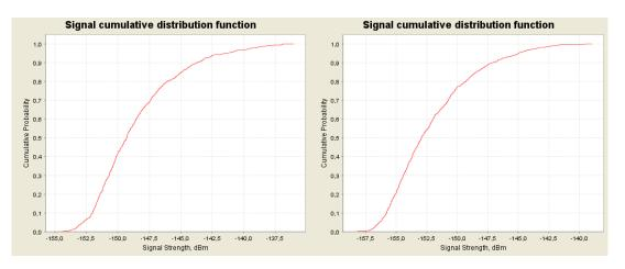
Figure 37: CDF graphs for the NCU (GSM) for 900 MHz at 8000 m (left) and 10000 m (right) above ground
