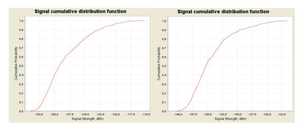
Figure 53: CDF graphs for the NCU (CDMA) for 450 MHz at 8000 m (left) and 10000 m (right) above ground
