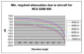
Figure 15: Attenuation requirements on signals to/from the radiating cable
