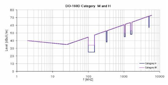
92: Limit line for emission of radio frequency energy according to category M and H
