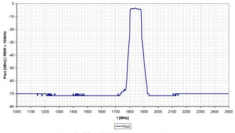
Figure 98: GSM 1800 output spectrum wideband
