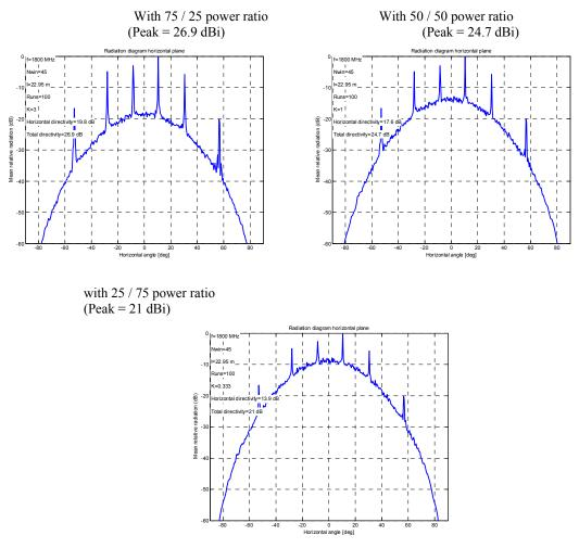
Figure 82 Azimuth plots of aircraft aperture and array gain determined by a Rician two-component model for different coherent/random power ratios
