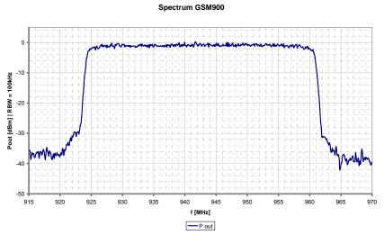
Figure 93:GSM 900 output spectrum narrow band
