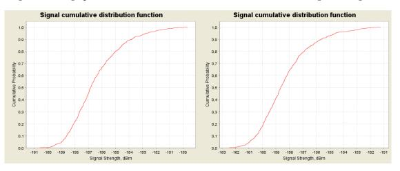
Figure 69: CDF graphs for the ac-MS for 1800 MHz at 8000 m (left) and 10000 m (right) above ground
