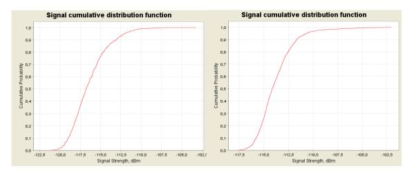
Figure 58: CDF graphs for the multiple NCU (GSM) for 900 MHz for normal busy (left) and extreme busy (right) cases
