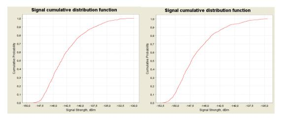
Figure 47: CDF graphs for the NCU (GSM) for 1800 MHz at 8000 m (left) and 10000 m (right) above ground
