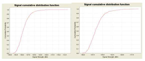
Figure 56: CDF graphs for the multiple NCU (GSM) for 900 MHz for normal busy (left) and extreme busy (right) cases
