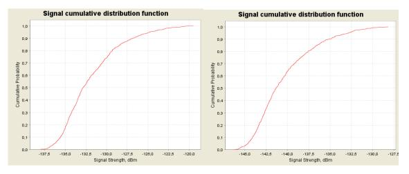
Figure 36: CDF graphs for the NCU (GSM) for 900 MHz at 3000 m (left) and 5000 m (right) above ground
