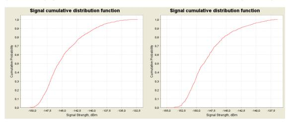
Figure 51: CDF graphs for the NCU (UMTS) for 1800 MHz at 8000 m (left) and 10000 m (right) above ground
