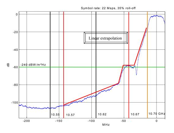
Figure 6: Out-of-band emission mask of digitally modulated FSS signal
