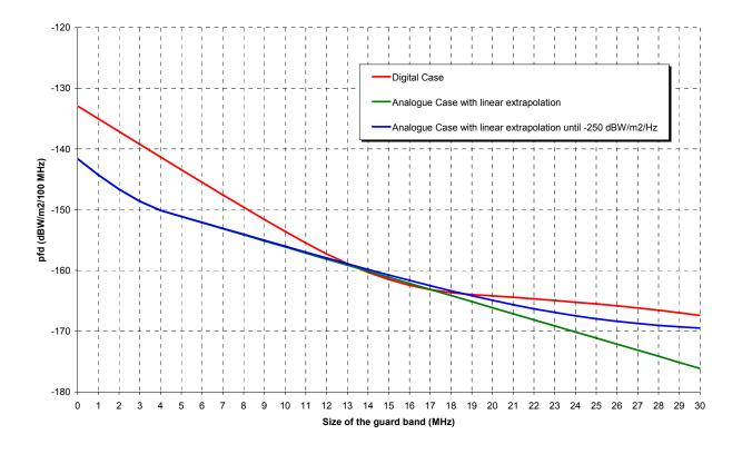
Figure 8: Evaluation of guard band necessary to protect the RAS
