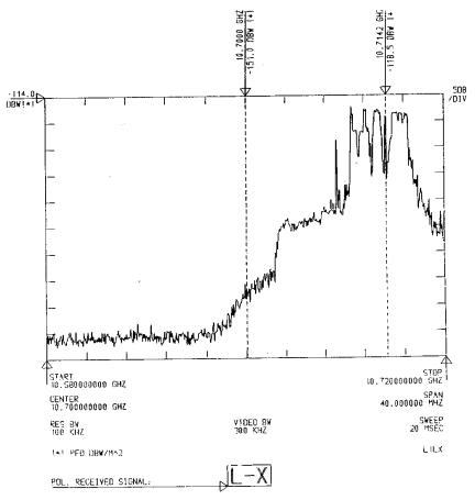
Figure 3: Measurement of interference source conducted at Leeheim monitoring station (1995)
