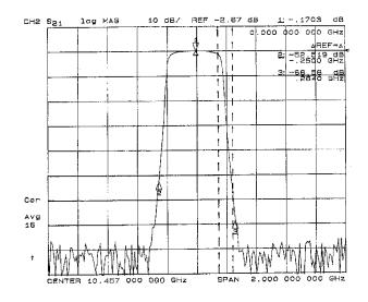
Figure 5: Filter attenuation curve of the employed band-rejection filter
