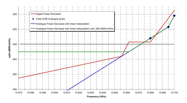
Figure 7: OOB emissions from various FSS signals into the frequency band below 10.7 GHz
