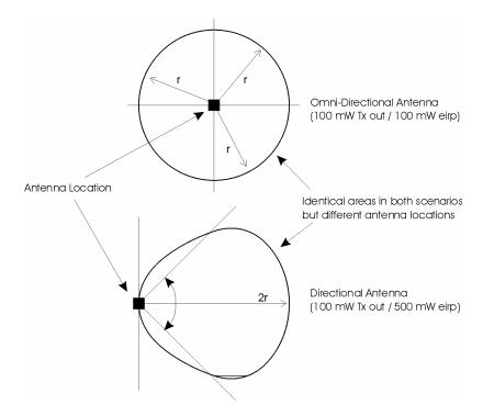
Figure 1: Increase of Operating Distance by Using a Directional Antenna
