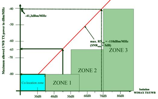
Figure 8: Maximum UWB Tx Power at Downlink AMC Inside Cell
