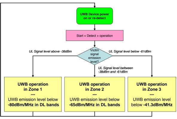
Figure 2: DAA flow chart revision in the frequency band 3.4-4.2 GHz
