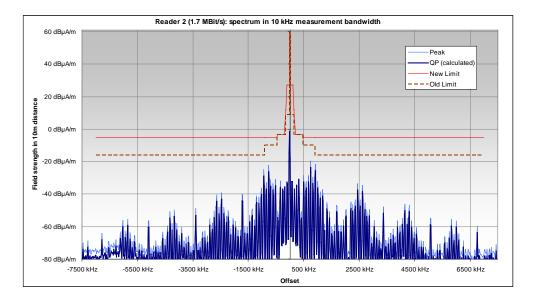
Figure 13: QP spectrum of Reader 2 and spectrum masks far from the carrier
