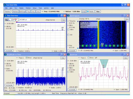
Figure 18: Time analysis of the Reader 2 signal for a 1 s time interval
