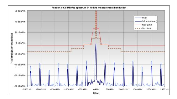
Figure 14: QP spectrum of Reader 3 and spectrum masks close to the carrier
