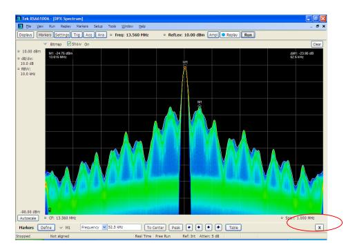
Figure 8: DPX spectrum of Reader 1 (high power, low bandwidth)
