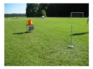
Figure 22: Electrical monopole measurement antenna
