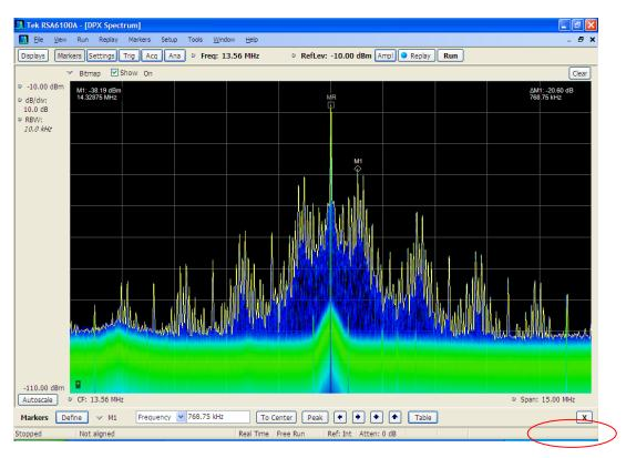
Figure 9: DPX spectrum of Reader 2 (low power, 1.7 MBit/s)
