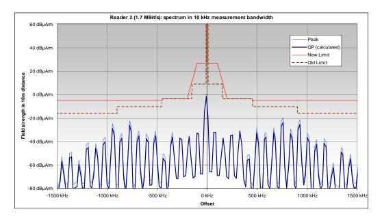
Figure 12: QP spectrum of Reader 2 and spectrum masks close to the carrier
