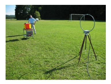
Figure 21: Magnetic loop measurement antenna
