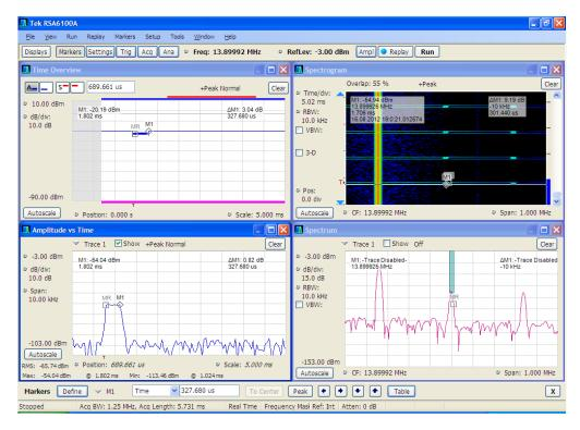
Figure 19: Time analysis of the Reader 3 signal for a 5 ms time interval
