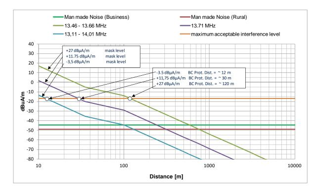
Figure 33: Magnetic field strength and protection distances for different emission levels of the TX mask (indoor operation)
