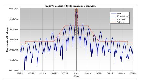
Figure 11: QP spectrum of Reader 1 and spectrum masks
