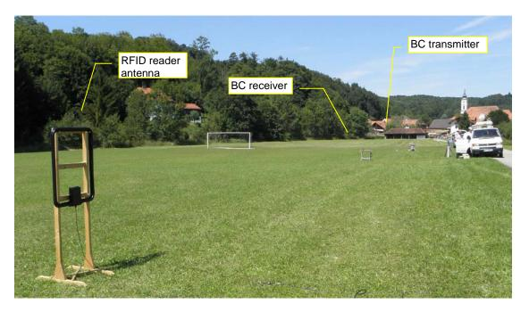
Figure 28: RFID reader antenna at 30 m distance to victim receiver
