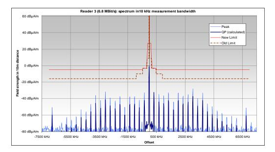
Figure 15: QP spectrum of Reader 3 and spectrum masks far from the carrier
