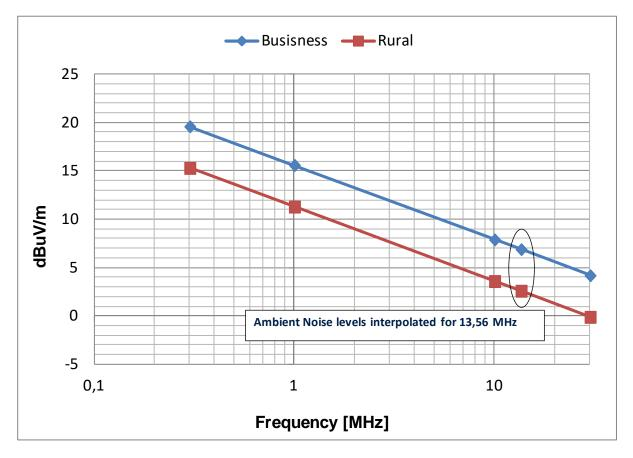
Figure 31: Slope of Frequency dependent man-made noise level to determine noise levels at 13.56 MHz
