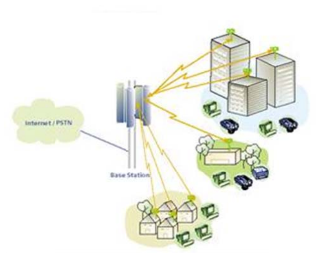
Figure 7: Typical BFWA P-MP deployment scenario (from ECC Report 068 [16])
