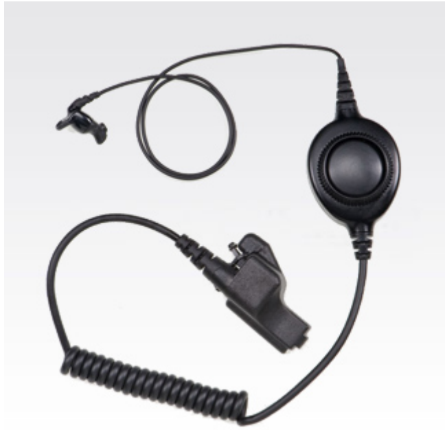
Figure 44: In ear bone conduction microphone-receiver
