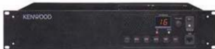
Figure 37: Talkback rack equipment
