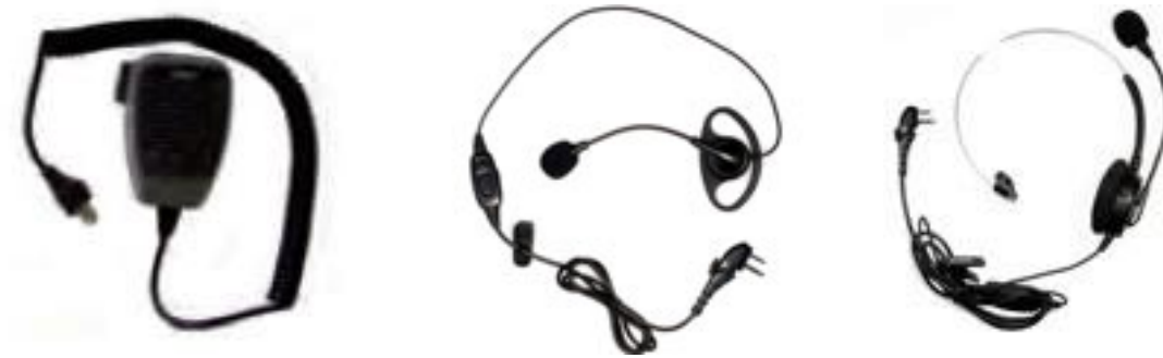
Figure 42: Remote microphone (on the left) headsets with a boom microphone (centre and on the right)
