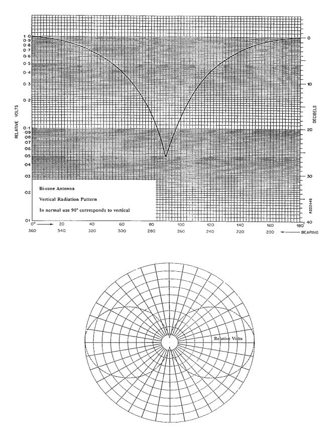
Figures 7 & 8: Radiation Pattern of Bicone Antenna
