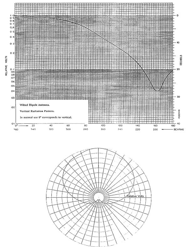
Figures 1 & 2: Radiation Pattern of Wilted Dipole Antenna
