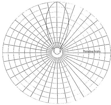
Figures 11 & 12: Radiation Pattern of Disk Yagi Antenna
