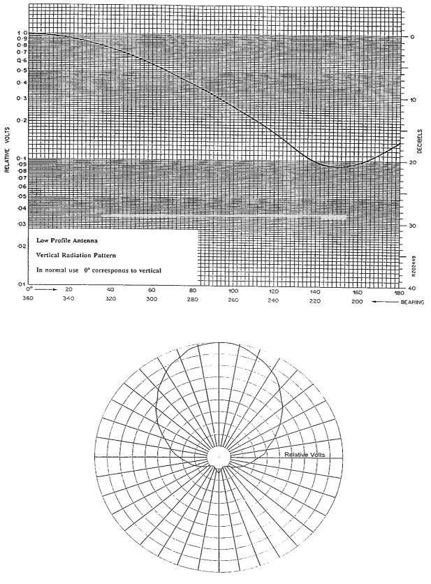
Figures 3 & 4: Radiation Pattern of Low Profile Antenna
