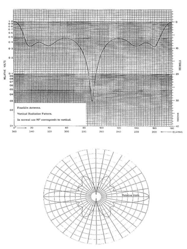
Figures 5 & 6: Radiation Pattern of Franklin Antenna
