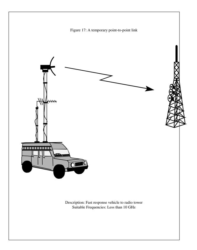
If transmit and receive terminals are not line of sight a mid-point may be necessary.
