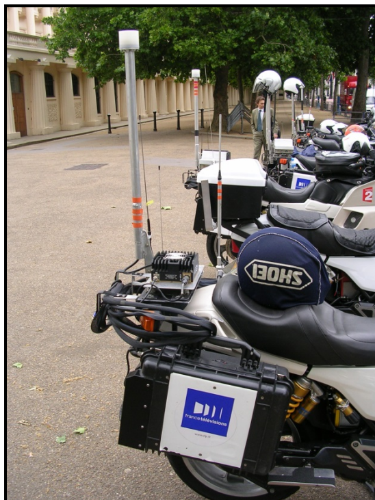
Figure 5: Mobile vehicular video link
