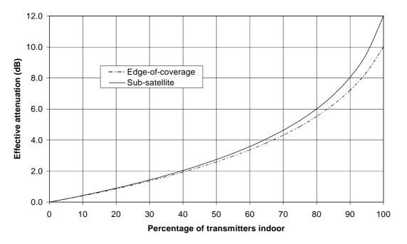
Figure 5 - Variation of effective attenuation with percentage of transmitters indoor
