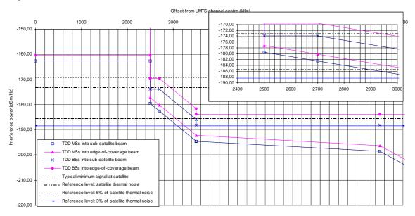
Figure 4 - Interference power at a satellite receiver from the TDD mode of terrestrial UMTS used to provide outdoor coverage
