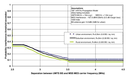
Figure 6 – Probability of MES receiver interference as a function of carrier frequency separation
