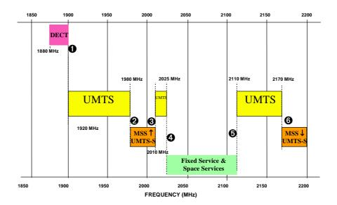
Figure 1 - European frequency plan for the 2 GHz band
