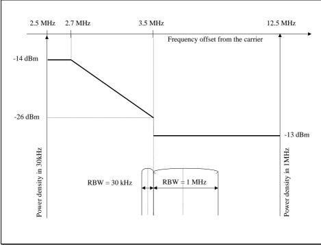
Figure A2 – BS Spectrum emission mask measured in 30 kHz bandwidth
