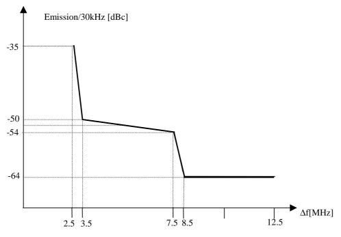
Figure A1 - UMTS Mobile Station (or UE : User Equipment) spectrum mask
