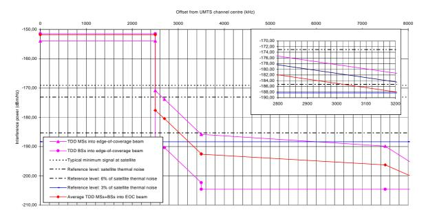
Figure 3 - Interference power at a satellite receiver from the TDD mode of terrestrial UMTS used to provide limited area indoor coverage
