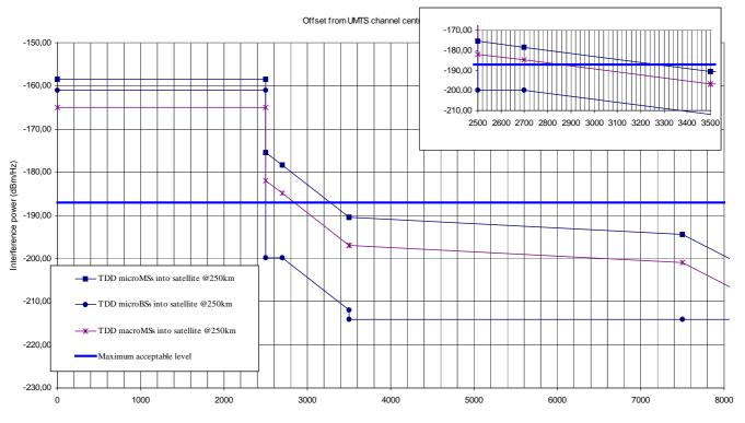
The figure below compares the aggregated received power at the spacecraft antenna as a function of the frequency offset.
