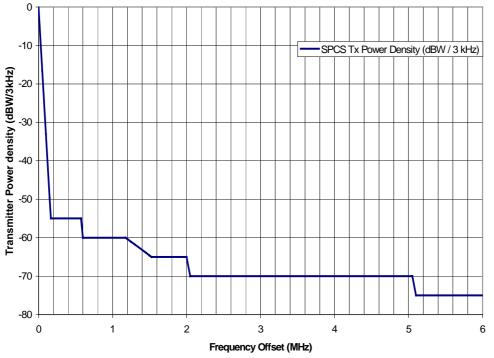
Figure A5 - 2 GHz S-PCN out-of-band mask
