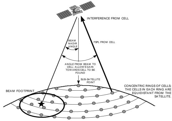
Figure B1 : Interference Calculation Methodology
