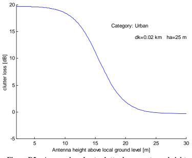
Figure D2 – Average loss due to clutter loss vs antenna height
