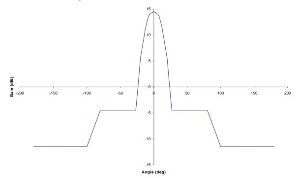
Figure A4 – Base Station antenna pattern
