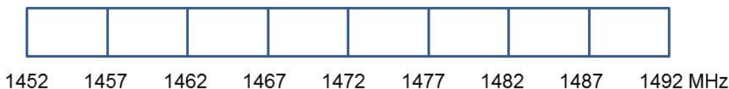
Figure 7: Band plan option B for 1452-1492 MHz band based on 5 MHz block size
