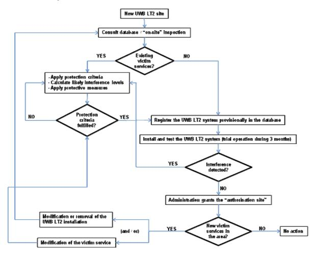
Figure 1: Flowchart describing the coordination/registration mechanism
