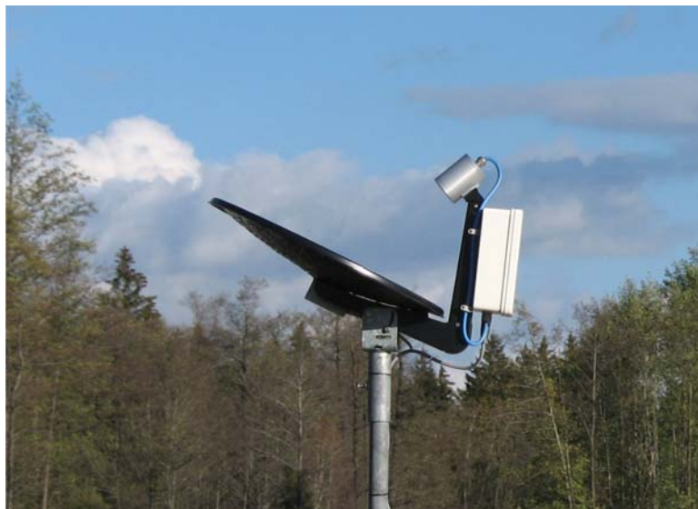
Figure 1: Micro Rain radar with vertically pointing offset parabolic dish antenna
