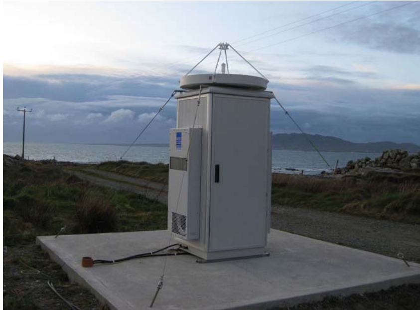
Figure 2: Cloud radar with fixed vertically pointing parabolic dish antenna
