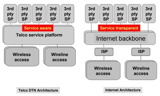
Figure 12: Comparison of the telco and Internet architectures
