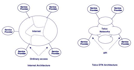
Figure 7: Comparison of telco DTN architecture and the Internet
