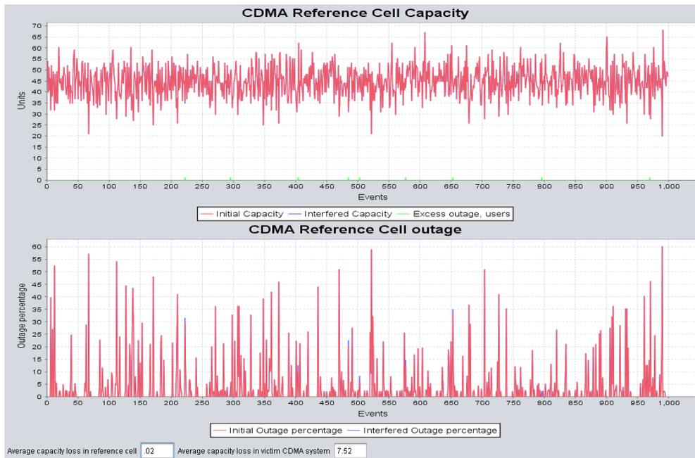
**Figure 7: Results of simulated interference scenario LP-AMI-P to IMT-2000 downlink**
