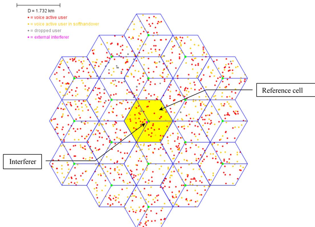
**Figure 6: Single snapshot of simulated interference scenario LP-AMI-P to IMT-2000 downlink**
