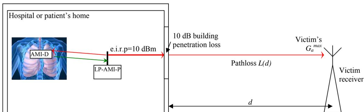
**Figure 1: Considered critical impact scenario for LP-AMI operation**
