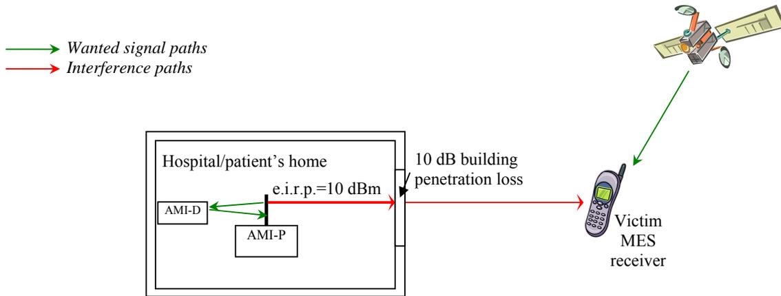
**Figure 2: Interference scenario LP-AMI vs MSS (Globalstar)**
