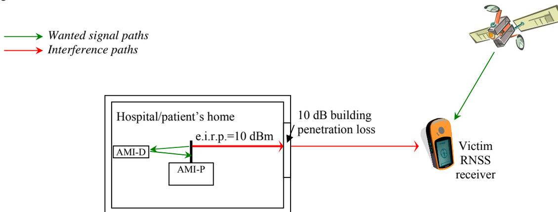
**Figure 9: Interference scenario LP-AMI vs. RNSS (Galileo evolution)**
