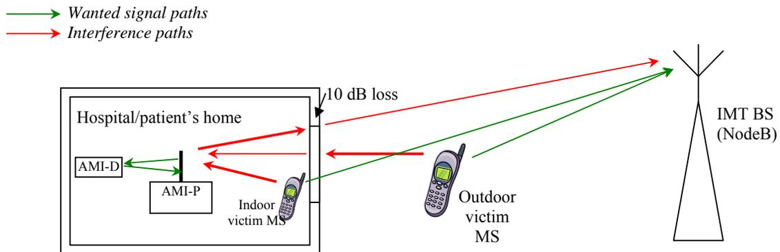
**Figure 5: Interference scenarios LP-AMI vs IMT-2000 Uplink**
