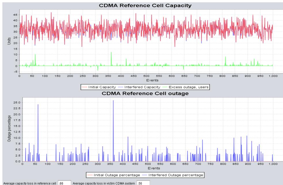
**Figure 8: Results of simulated interference scenario LP-AMI-P to IMT-2000 downlink**
