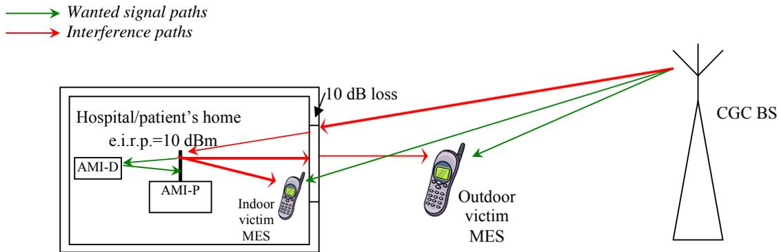
**Figure 3: Interference scenarios LP-AMI vs MSS CGC**
