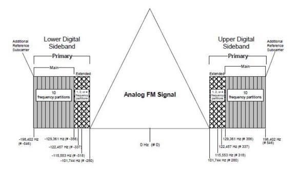
Figure A1-3: The graph indicates the extended-hybrid mode (MP11) configuration. A different hybrid configuration can be used in the same example, using MP1 mode by eliminating the Extended Hybrid carriers. (see Figure A1-5)
