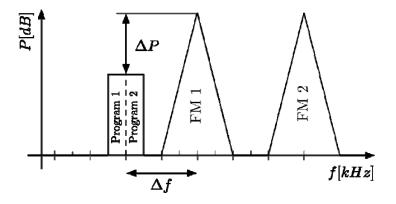
Figure A1-2: Example configuration with 2 FM Stations and DRM robustness mode E
