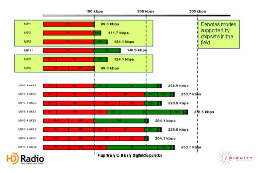
Figure A1-5: The graph indicates the various operating modes and their bit-rate throughputs. These modes are user selectable, and may be changed at any time desired
