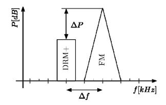
Figure A1-1: Example configuration for DRM robustness mode E and FM signal
