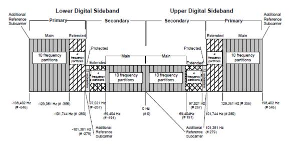
Figure A1-4: The graph represents one configuration of the all-digital operation. See Figure A.1-5 for throughput options
