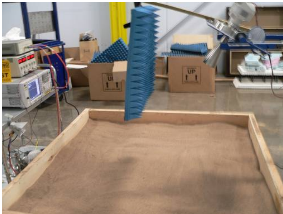
(b) Figure A2.2: Measurement set-up for evaluating reflection properties of fine dry sand: (a) functional scheme, (b) photograph of a practical set.
