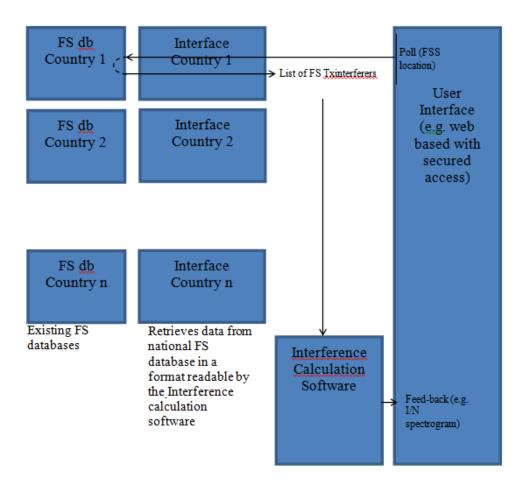
Figure 6: Detailed diagram
