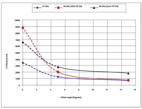
Figure 10: Required separation distances for Scenario 1: FLANE Tx main beam to PP FS Rx as a function of offset angle between the links
