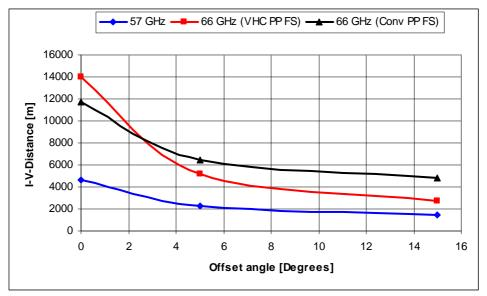
Figure 18: Required separation distances for scenario 1 : FLANE 55dBm Tx main beam into PP FS (VHC and Conv.) Rx as a function of offset angle between the links (see Figure 10 for comparison with an e.i.r.p of 40 dBm).
