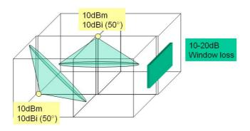
Figure 1: Illustration of indoor WLAN deployment
