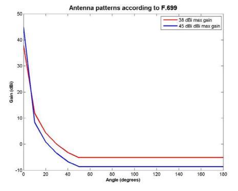
Figure 21: Antenna pattern according to ITU-R F.699 for a nominal gain of both 38 and 45 dBi.
