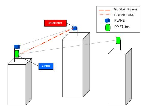
Figure 6: Scenario 1: FLANE Tx main beam to PP FS Rx side lobes
