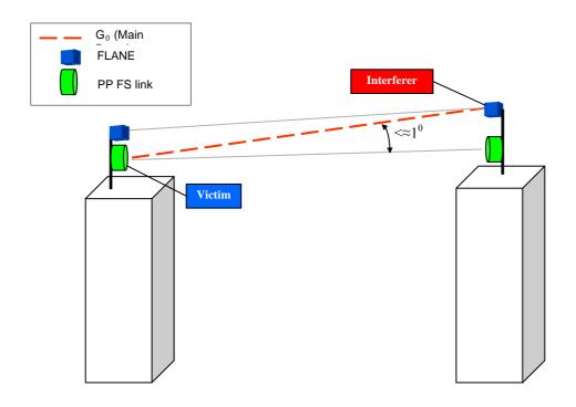
Figure 7: Scenario 2: FLANE Tx main beam to PP FS Rx main beam (co-located case)
