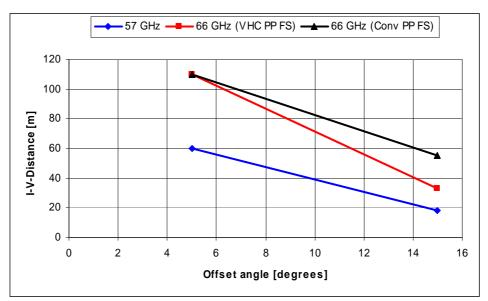
Figure 12: Required separation distances for Scenario 4: WLAN Tx main beam to PP FS as a function of offset angle between the links
