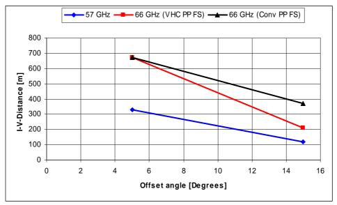
Figure 11: Required separation distances for Scenario 3: WPAN Tx main beam to PP FS Rx as a function of offset angle between the links
