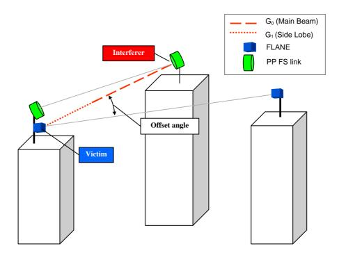
Figure 13: Scenario 5: PP FS Tx main beam into FLANE Rx side lobes
