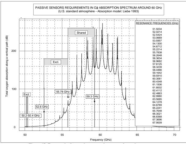
Figure 17: Frequencies for passive sensors in oxygen absorption spectrum
