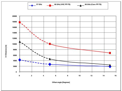
Figure 14: Required separation distances for Scenario 5: PP FS Tx main beam into FLANE Rx as a function of offset angle between the links
