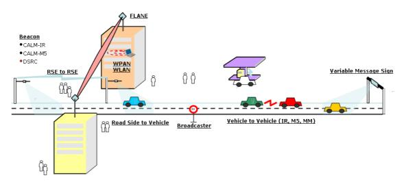
Figure 5: Example of ITS system deployment scenario, with FS links used in ITS backbone (RSE to RSE)
