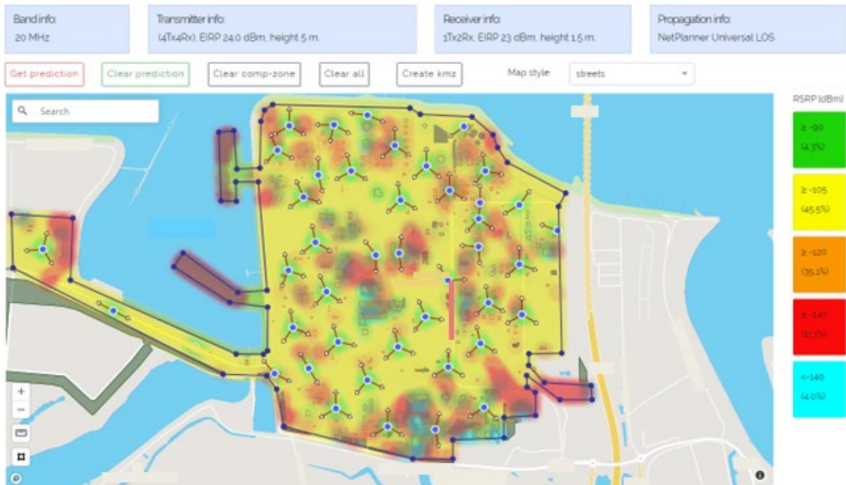
Figure 11: Simulated received signal strength (RSRP) of a local area network deployment as per the parameters of deployment Scenario 4
