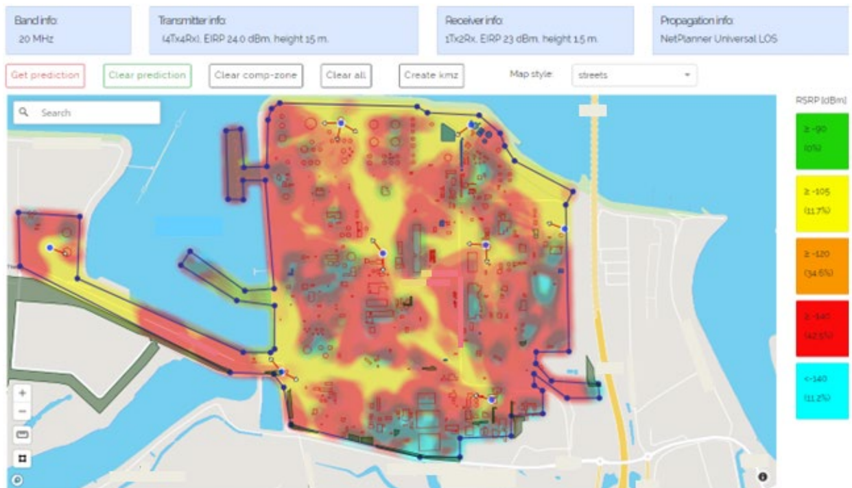
Figure 9: Simulated received signal strength (RSRP) of a local area network deployment as per the parameters of deployment Scenario 2
