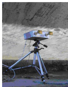
Figure A.2: GBSAR system configuration for structure monitoring applications
