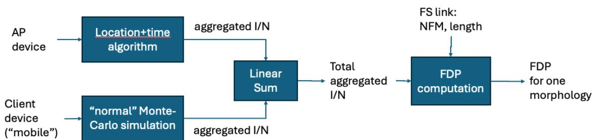
**Figure 37: Complete simulation process to derive the FDP(%)**
