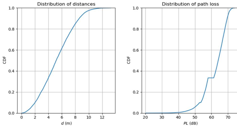
**Figure 136: Monte Carlo generated ECDF of distance  $d(\omega)$  and associated empirical CDF of transmission loss  $PL(\omega)$**
