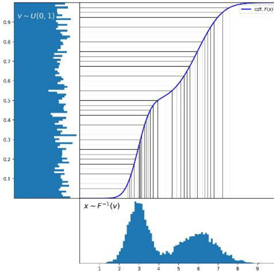
**Figure 131: The inverse sampling technique can be used to generate random numbers adhering to a given target probability distribution by using the inverse CDF (or an approximation of it) and utilising uniformly distributed random samples**
