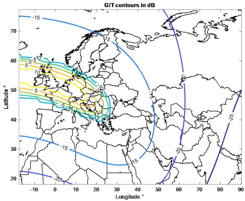
**Figure 100: Spot Beam (at 64° E) G/T contour**
