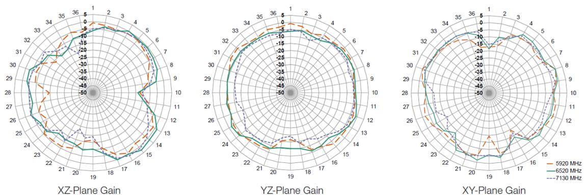
**Figure 22: Antenna diagrams from datasheet for ANT-W63-MON-ccc, Straight**
