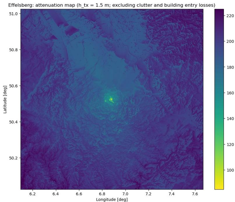
**Figure 118: Transmission loss (dB) for the area around the Effelsberg observatory, assuming 1.5 m transmitter heights (above ground)**
