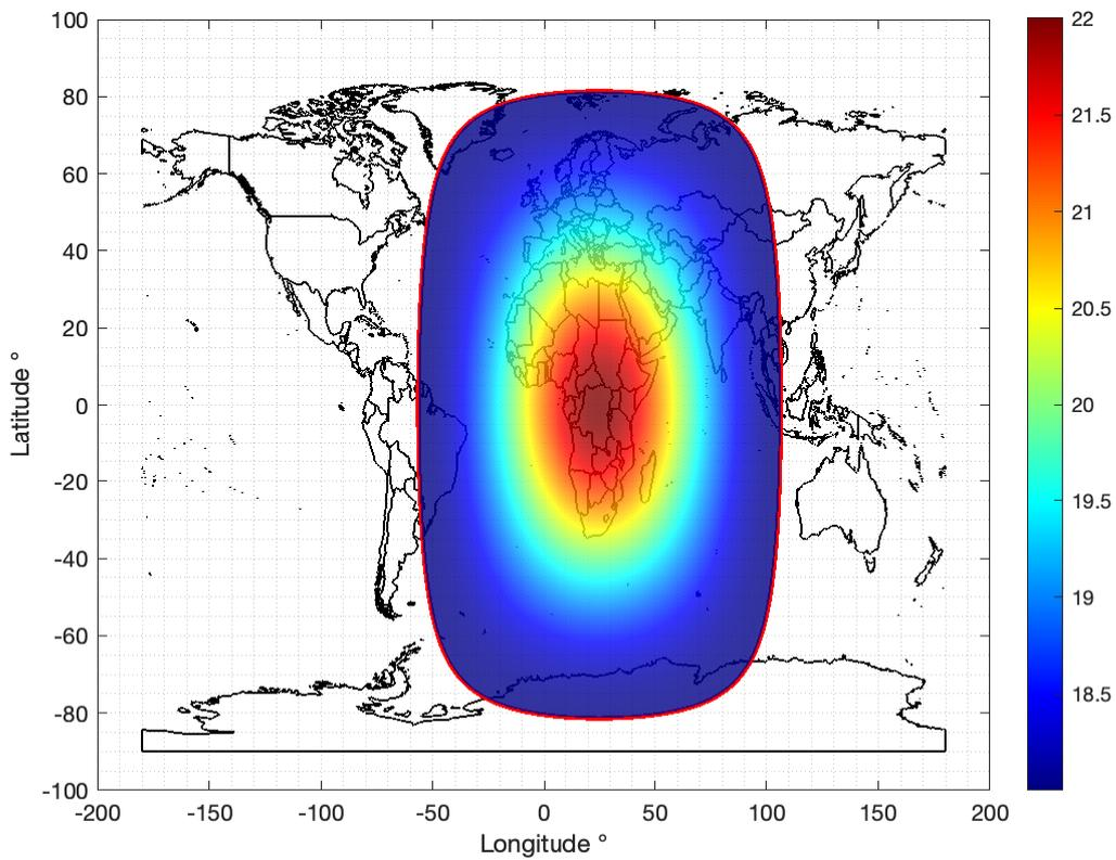
**Figure 98: Global Beam (at 25° E) G/T contour (top) and antenna receiver gain contour (bottom). Red curve is the zero-degree elevation visibility limit**
