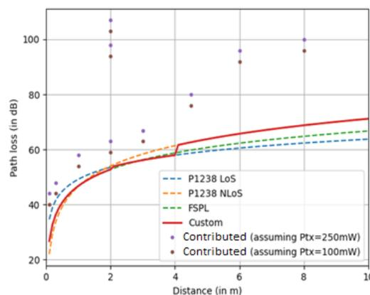
**Figure 135: Median transmission loss model used in this study, as a combination of FSPL, and site-general office model of Recommendation ITU-R P.1238-11**
