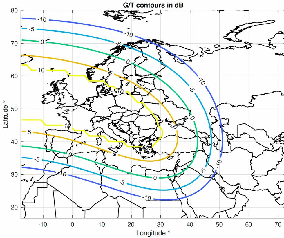
Figure 101: Spot Beam 2 (at 64° E) G/T contour
