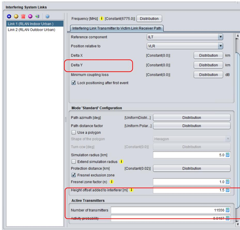
Figure 72: Indoor WAS/RLAN position locked after first event and active probability configuration
