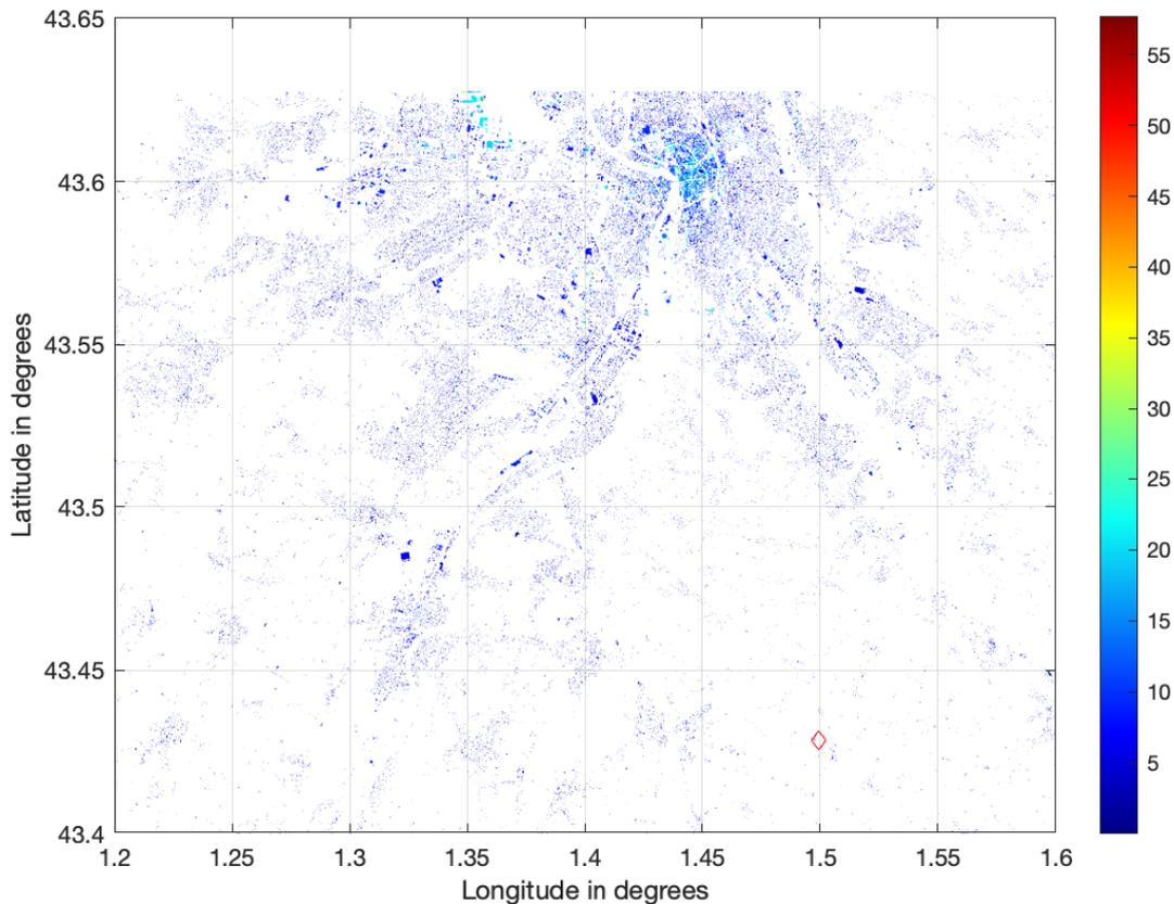
**Figure 114: Buildings positions and height around the ground station, the red diamond is the ground station's position**
