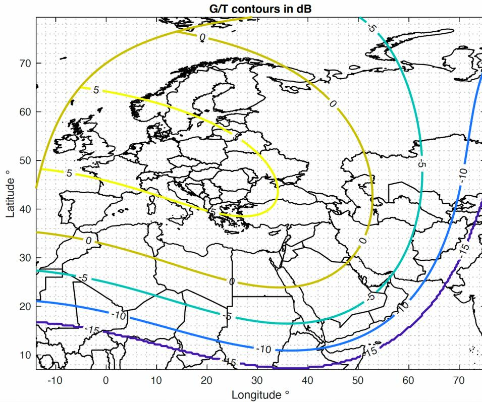
Figure 102: Zone Beam (at 64° E) G/T contour
