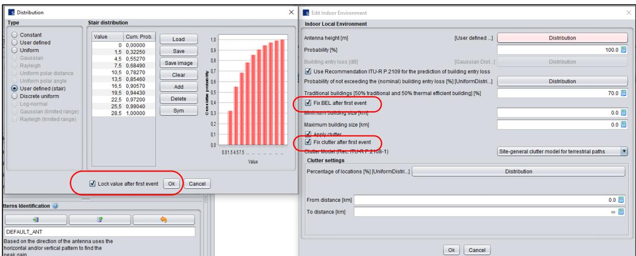
Figure 73: Indoor WAS/RLAN height, clutter loss and building entry loss locked after first event
