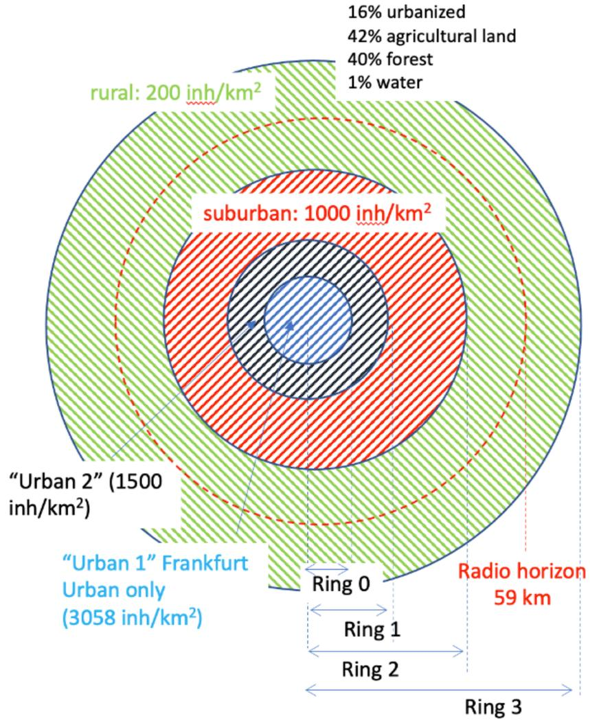
**Figure 27: Illustration of the generic ring model simulation derived from the Hessen state area (Frankfurt region) – The FS receiver is in the centre of the simulation area**
