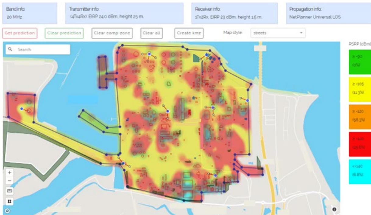
Figure 10: Simulated received signal strength (RSRP) of a local area network deployment as per the parameters of deployment Scenario 3
