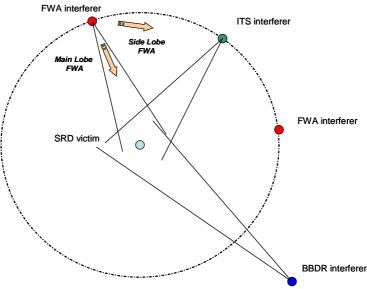
Figure 2: Aggregate impact around a SRD receiver
