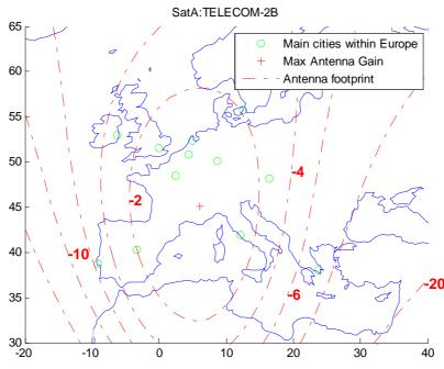
Figure 1: Antenna footprint for the satellite A
