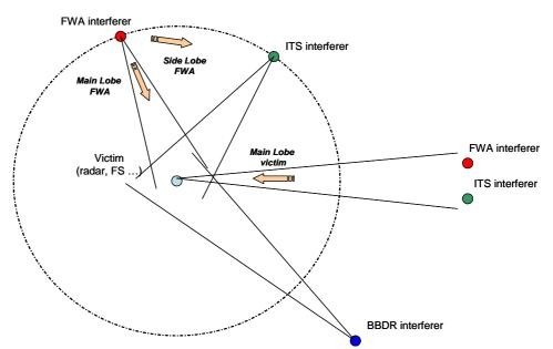
Figure 3: Aggregate impact around a long range (radar, FS...) receiver
