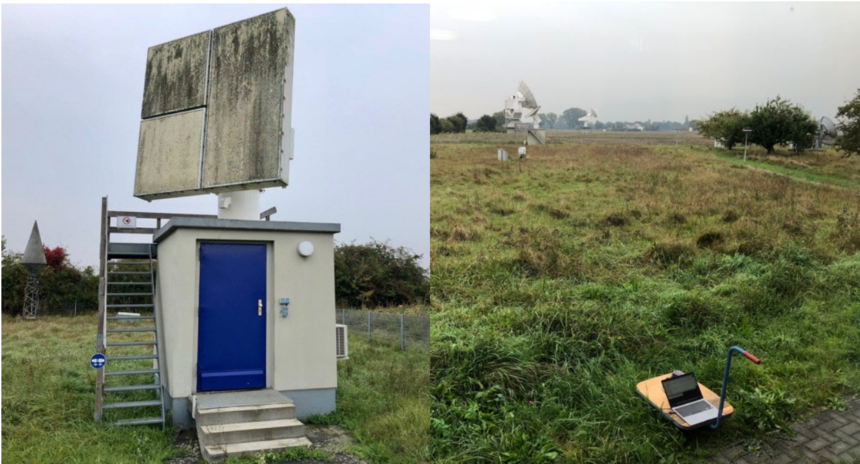
Figure 8: Leeheim Monitoring Station Left: Calibrated antenna to measure PFD value; Right: Lacuna Space user terminal and laptop placed on a cart to confirm reception of messages
