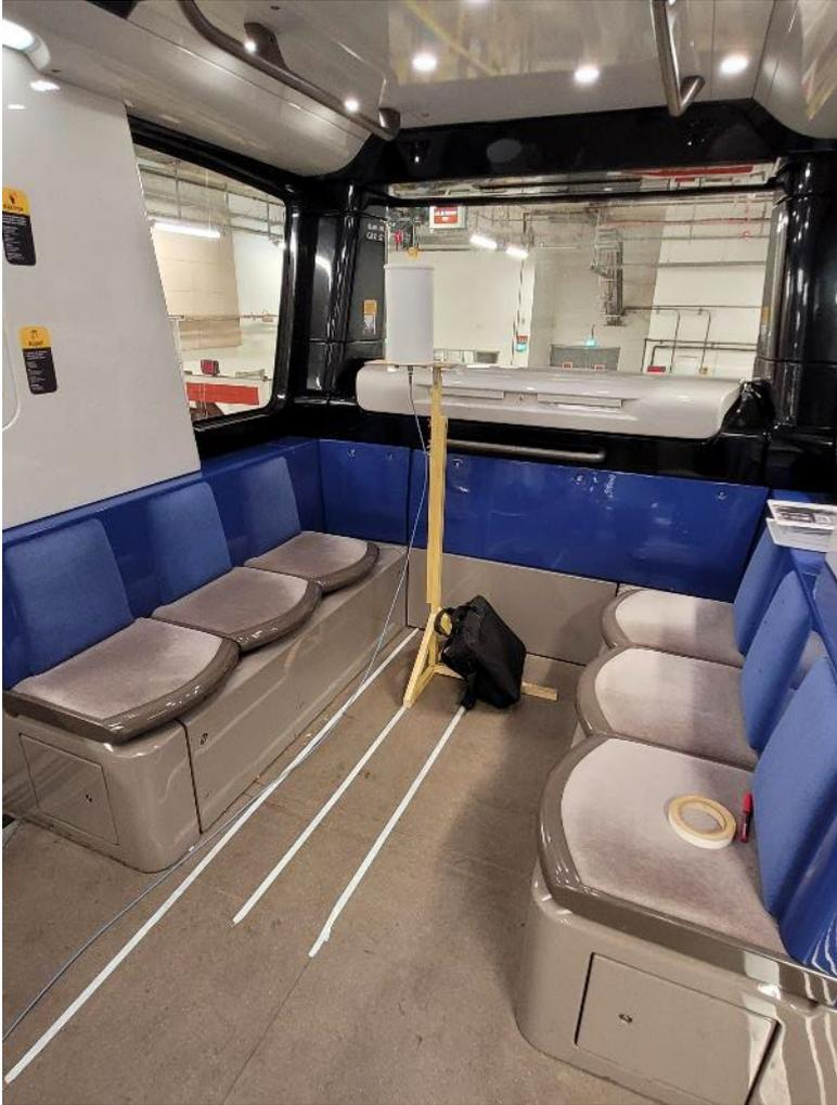
**Figure 34: Measurement grid and antenna**
