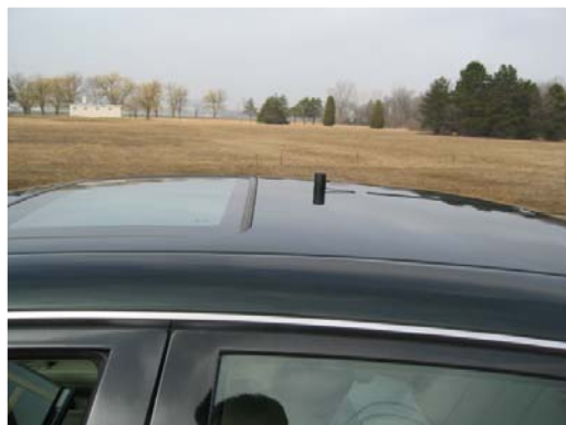
Figure 7: Ground-plane radio antenna with magnet roof mount (left side) and agreement of antenna’s pattern with the ITU F.1336 omni directional pattern (right side)
