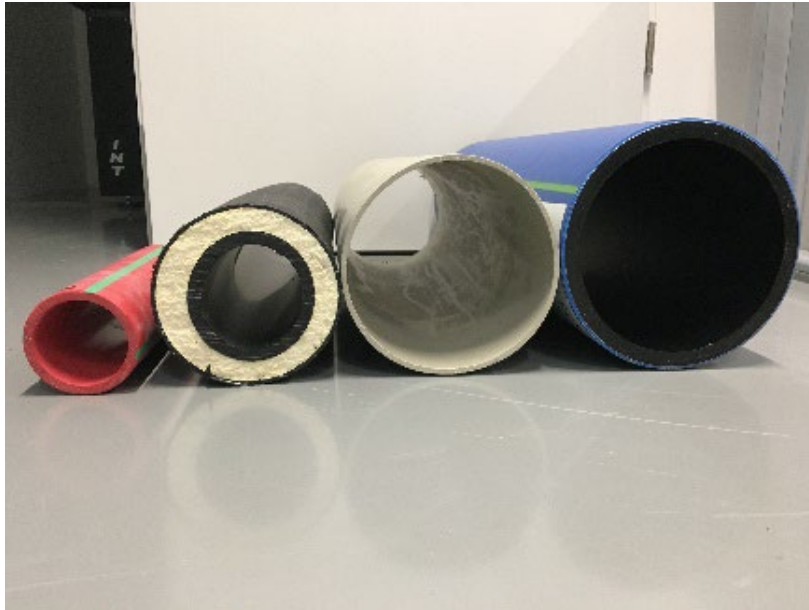
Figure 70: Standard pipes for gas, long-distance-heating, sheathing and fluid waste (left to right)
