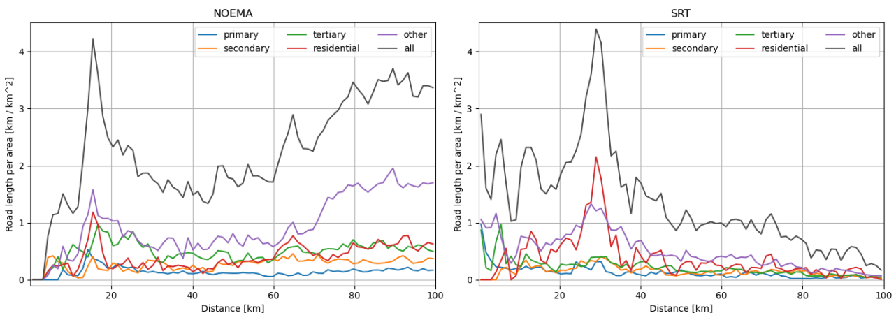
Figure 7: Road length per area per road type in distance bins around the RAS stations. Based on OpenStreetMap
