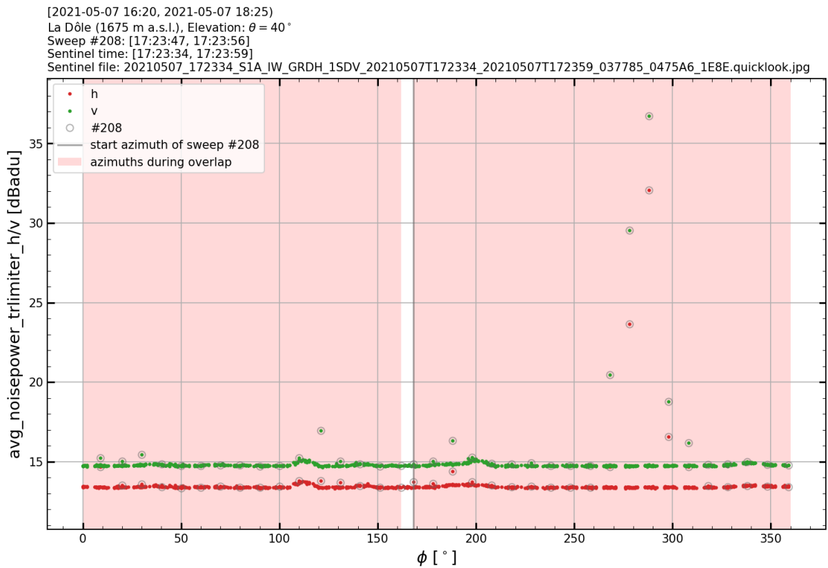
Figure 24: Measured noise power at elevation 40^\circ as a function of azimuth at ‘La Dôle’ on 7 May, 2021
