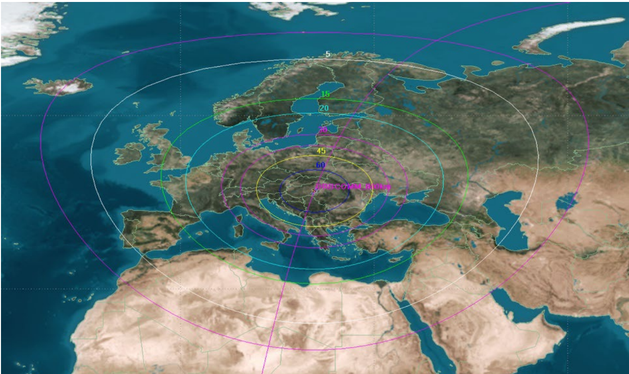
Figure 57: Illustration of the elevation-based division of the visibility area for an ORBCOMM satellite in transit at 800 km
