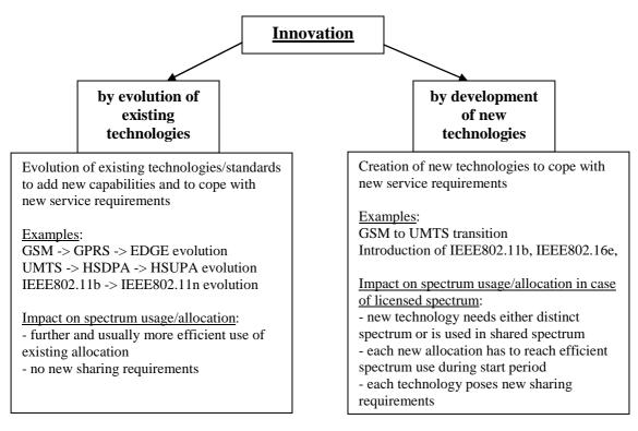
Figure 2: Types of innovation and their impact on spectrum usage/allocation
