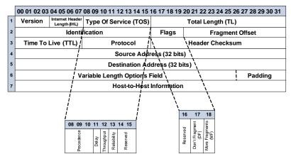
Figure 2: IPv4 Structure
