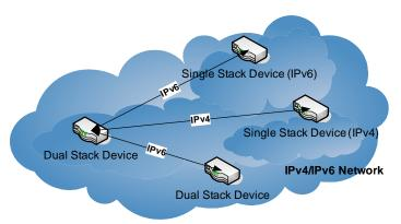
Figure 4: Dual stack operation
