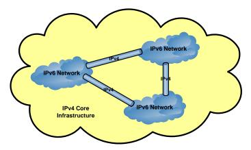
Figure 5: IPv4 Tunnelling with islands of IPv6 in and IPv4 core network (phase 1)
