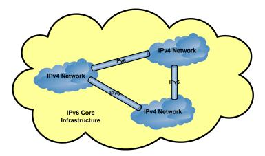
Figure 6: IPv6 Tunnelling with islands of IPv4 in and IPv6 core network (phase 2)
