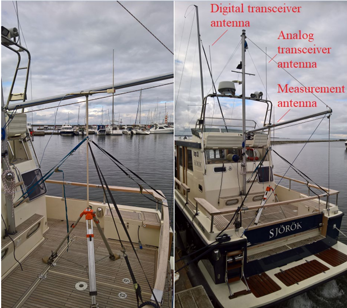
Figure 15: Antennas installed on a vessel
