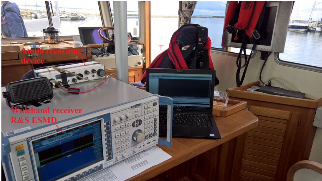
Figure 16: On-board measurement instrumentation Rohde & Schwarz
