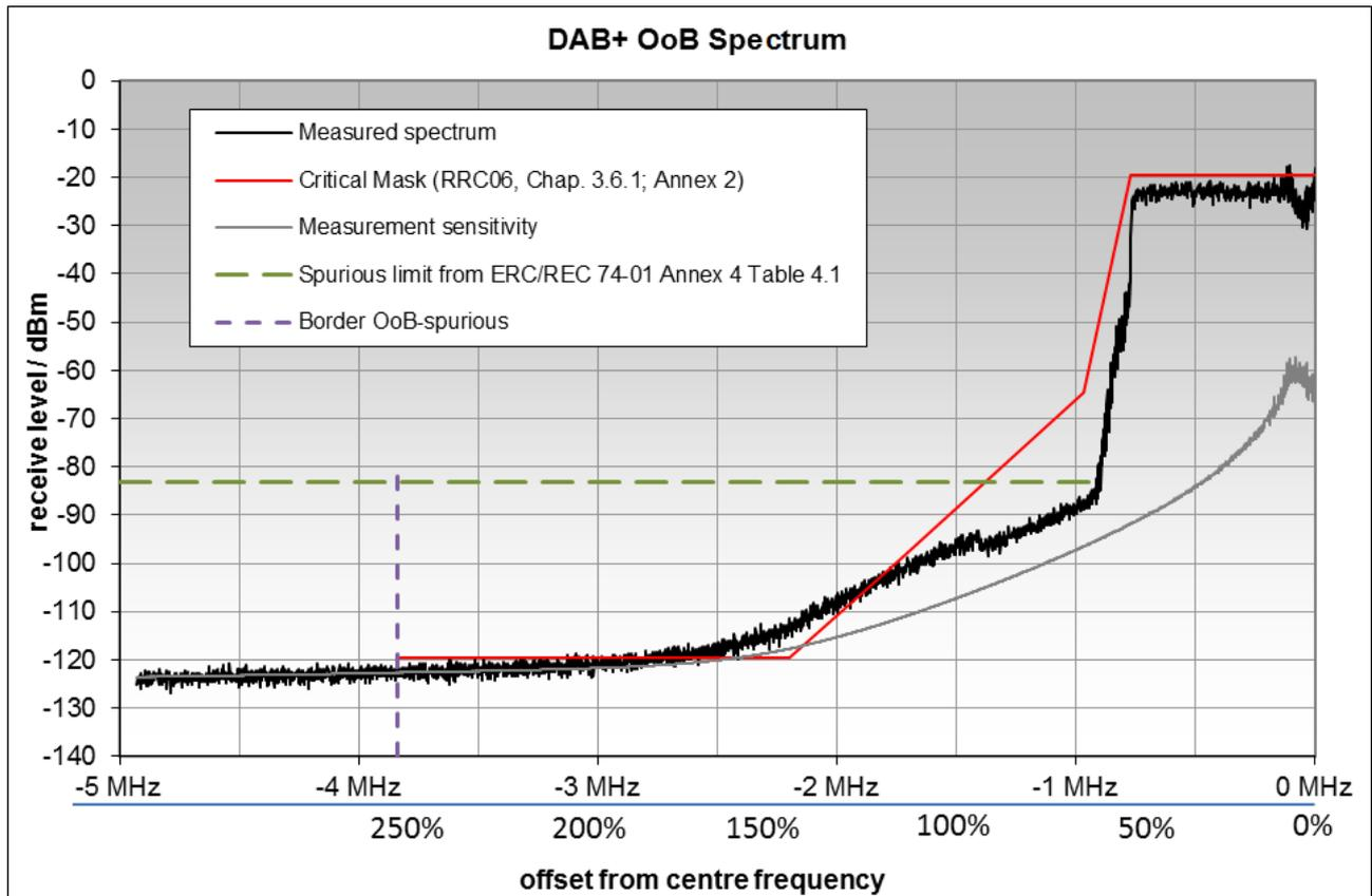
**Figure 2: OoB measurements from a DAB+ transmitter**
