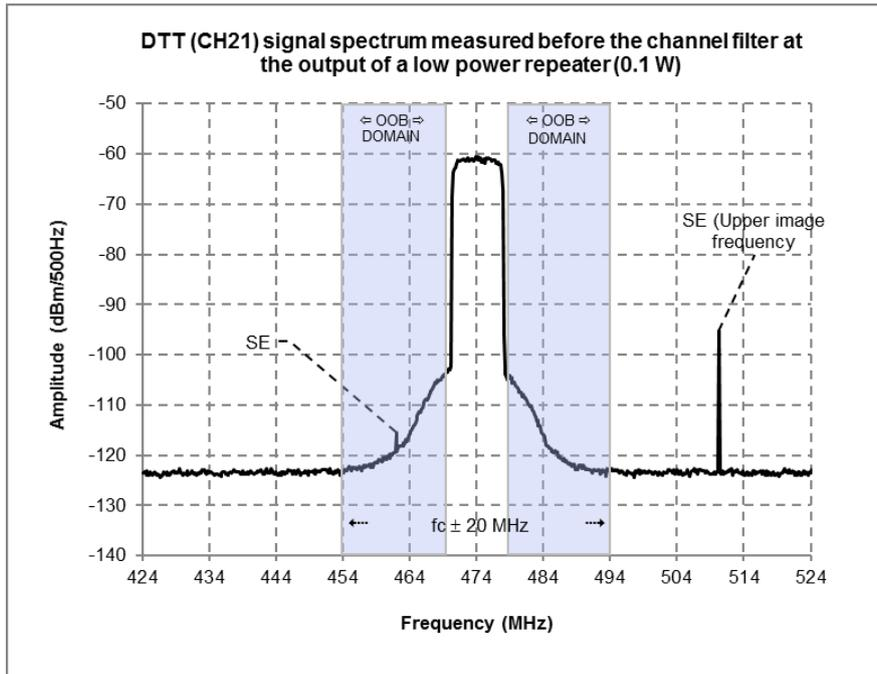
Figure 41: DTT Ch21 signal spectrum at the output of a low power repeater - 424-524 MHz
