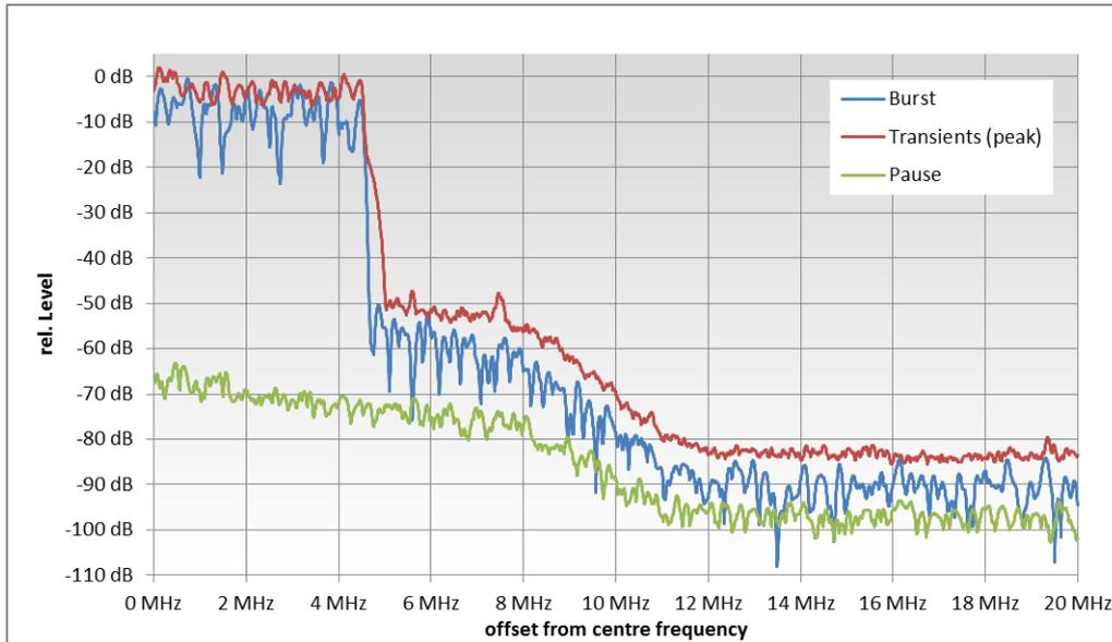
**Figure 46: LTE800 BS: OoB emissions at different times**
