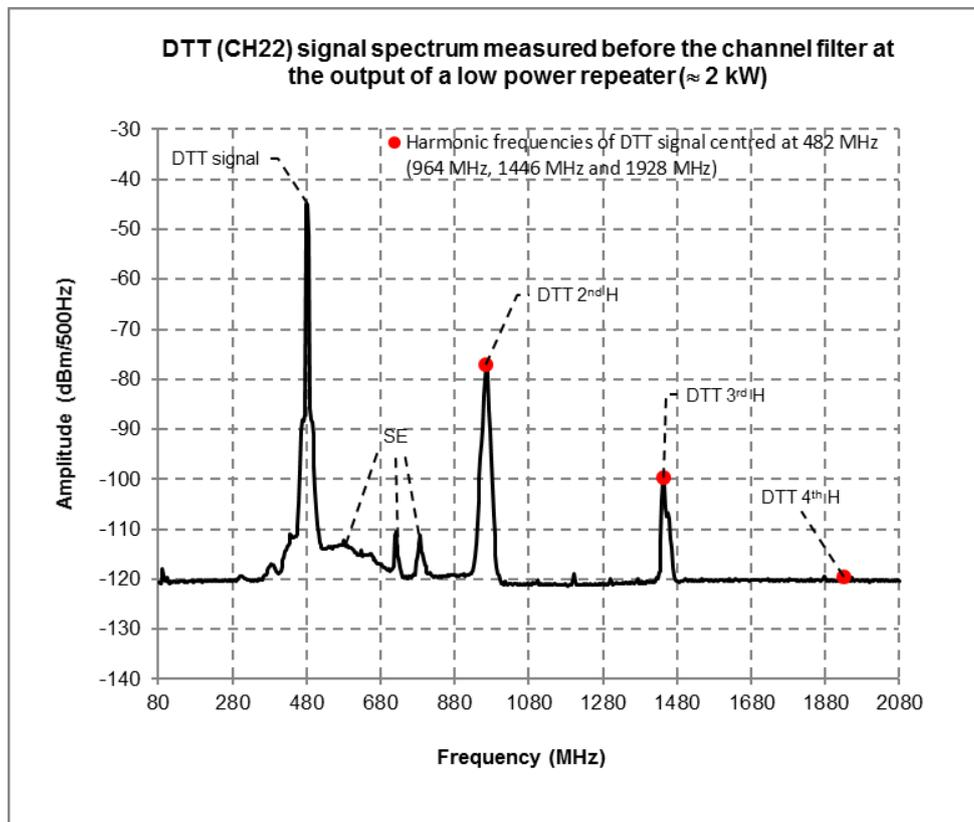
Figure 45: DTT Ch22 signal spectrum before the channel filter - 80-2080 MHz
