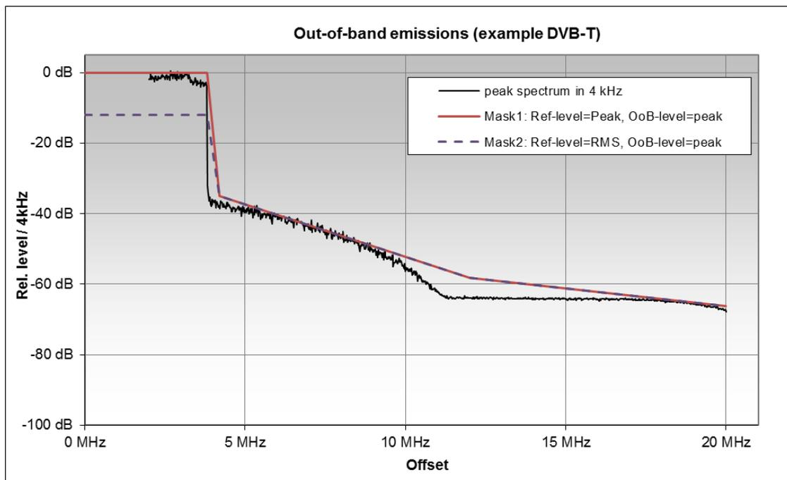
**Figure 52: Different mask definitions - an example (DVB-T OoB emissions)**
