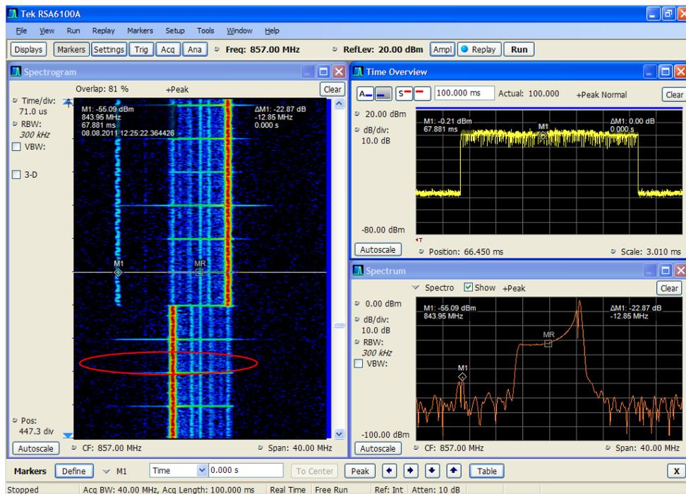
**Figure 47: Spectrum, power versus time and momentary spectrum at the time marked with a line (with points M1 and MR) in the spectrogram of a randomly selected LTE800 UE, high time resolution**
