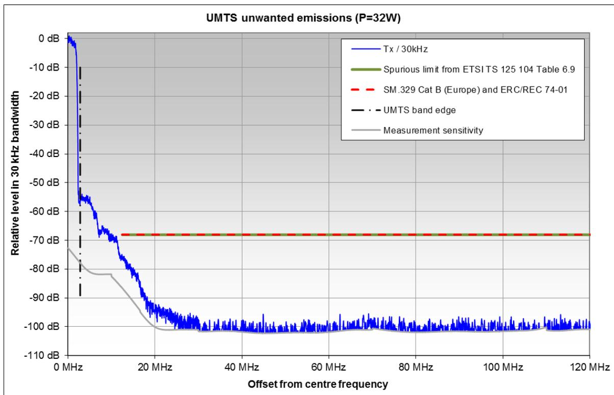
**Figure 29: Spurious emissions from a UMTS base station**
