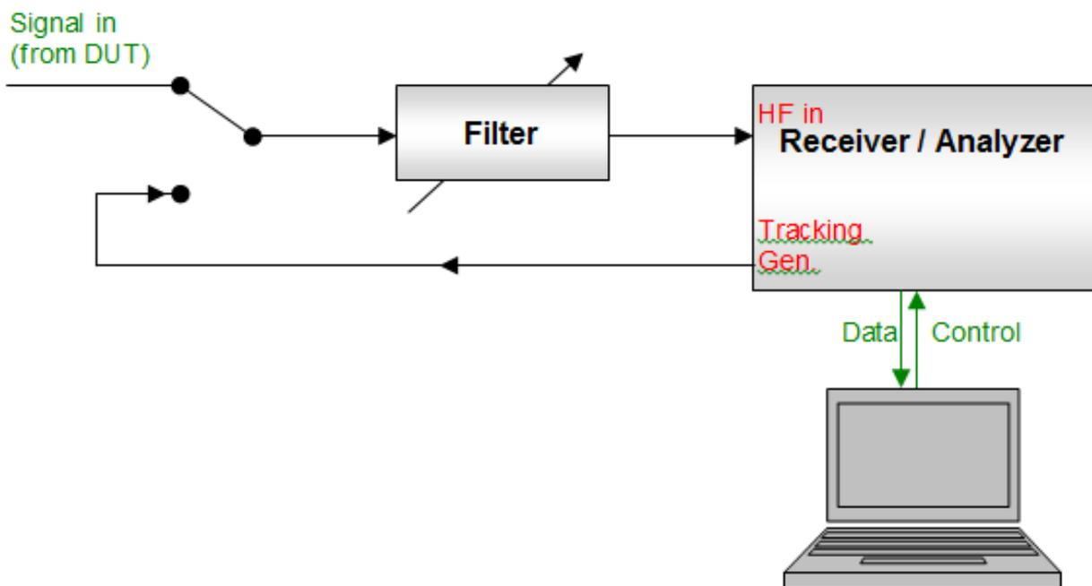
**Figure 50: Principle measurement setup Type 2**
