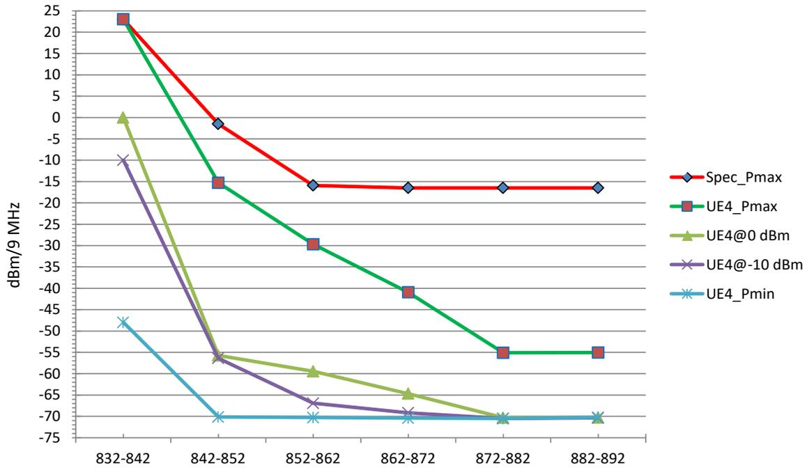
Figure 59: Measured UE#4 OOB Emissions (QPSK modulation, 50 RBs)
