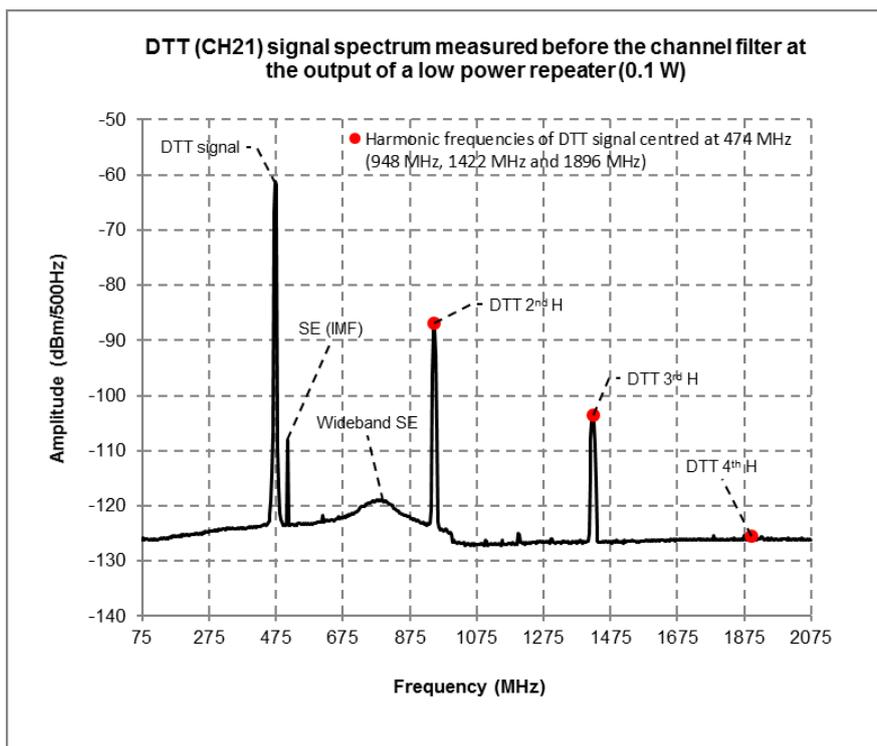
Figure 42: DTT Ch21 signal spectrum at the output of a low power repeater - 75-2075 MHz
