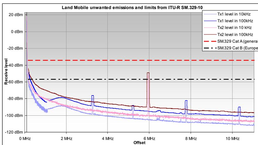
**Figure 48: Land Mobile spurious emissions from two different PMR transmitters (upper frequency range)**
