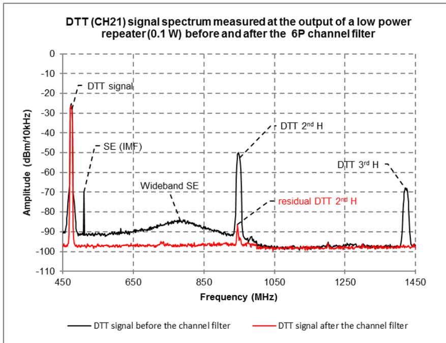
**Figure 43: DTT Ch21 signal spectrum before and after a 6-pole channel filter**
