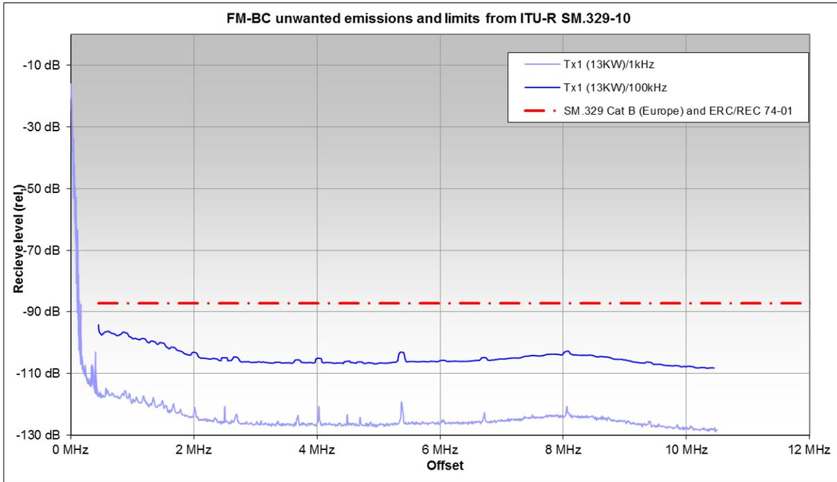
**Figure 68: Spurious emissions of a 13 kW FM broadcast transmitter (upper frequency range)**
