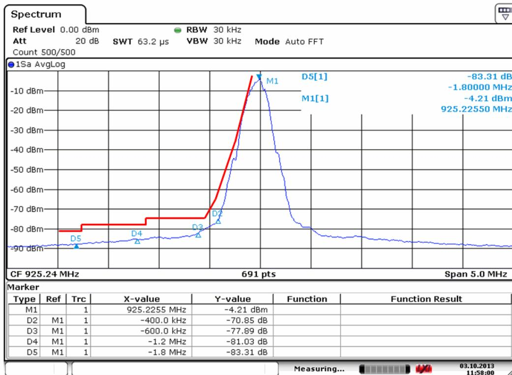
Figure 24: Measurement result of GSM900 base station test
