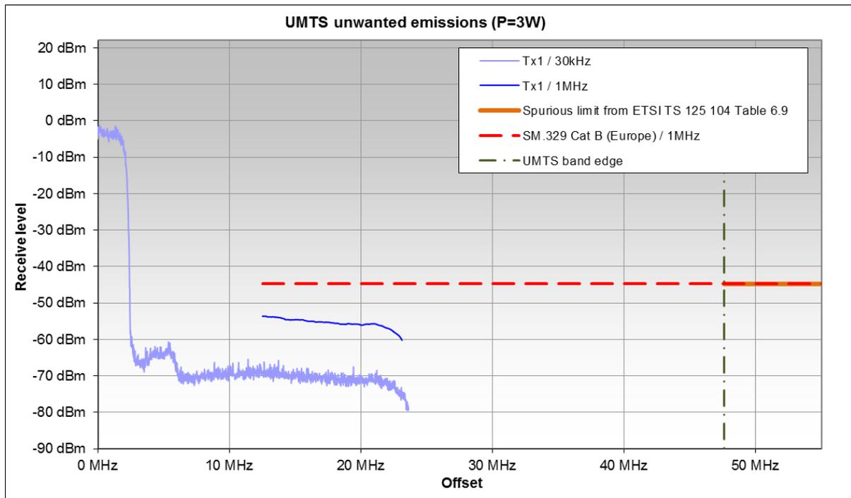
**Figure 63: UMTS spurious emissions (upper frequency range)**
