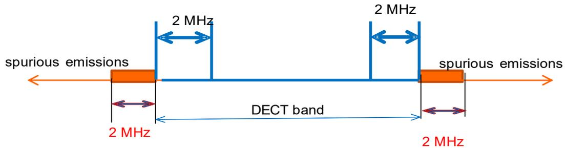
**Figure 55: Clarification on DECT OoB and spurious emissions terminology**
