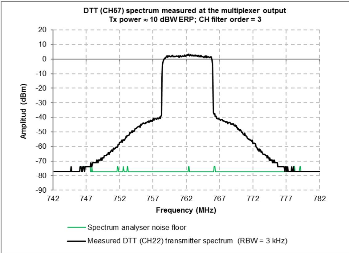
**Figure 5: Spectrum of a low power DVB-T transmitter**
