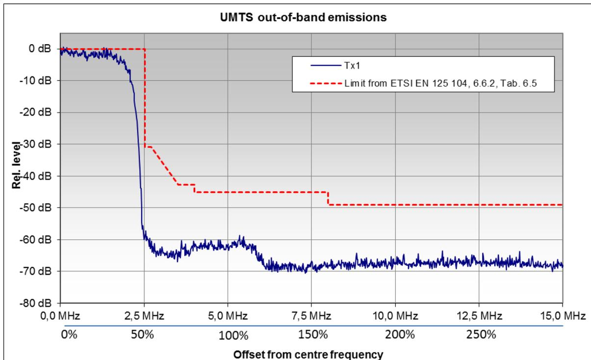
**Figure 28: OoB emissions from a UMTS base station**
