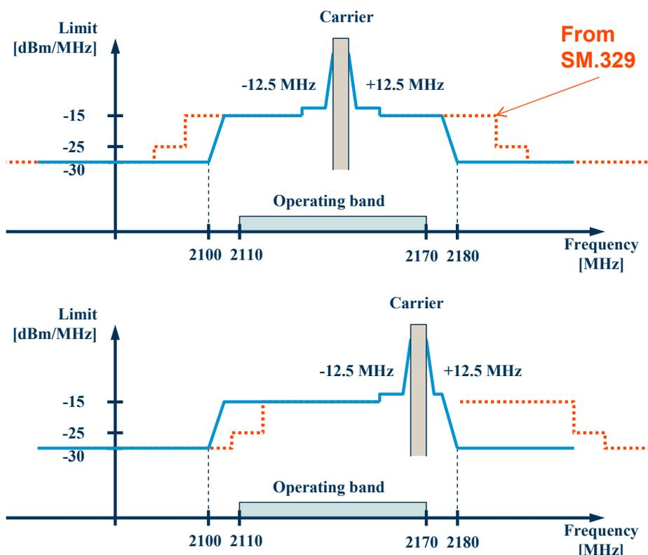
**Figure 53: UTRA Category B spurious emission limits for a single 5 MHz carrier in two example carrier positions. The dotted red line shows the relevant limits from ERC Recommendation 74-01 [2] and Recommendation ITU-R SM.329 [3]**
