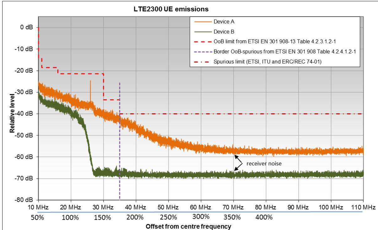
**Figure 23: Unwanted emission measurements of 2 LTE 2.3 GHz UEs (RMS power, resolution bandwidth = 10 kHz)**
