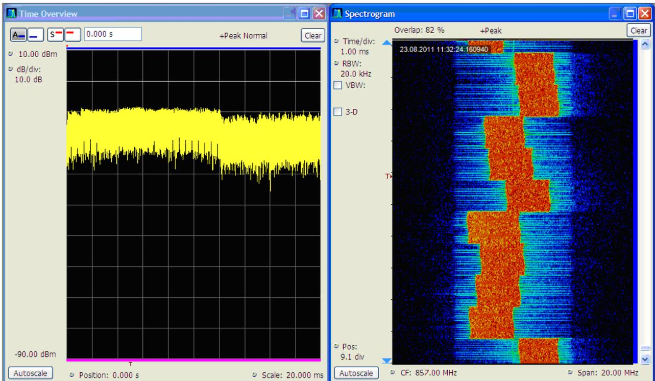
**Figure 56: Power versus time and spectrogram for signal UE2**
