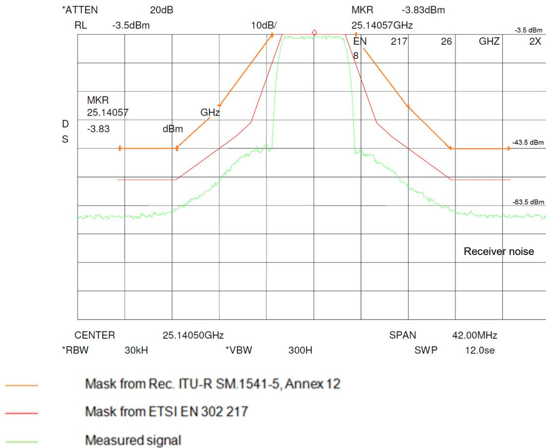
**Figure 65: 25 GHz Point to Point link unwanted emissions - Device B**
