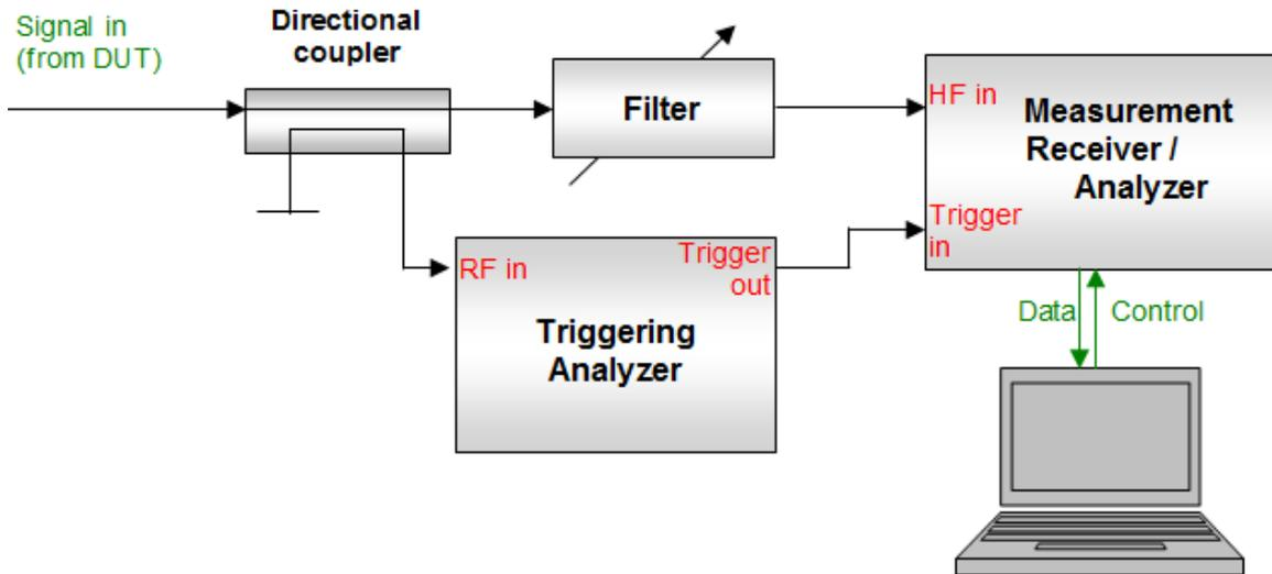
**Figure 51: Setup Type 3 for measurements of TDMA systems**
