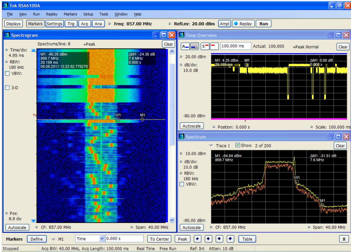
**Figure 58: Example of Out-of-Band emissions of a randomly selected LTE terminal. Spectrogram (left), power vs. time (upper right) and spectrum (yellow: whole acquisition time; orange: time instant marked with a line in the spectrogram)**
