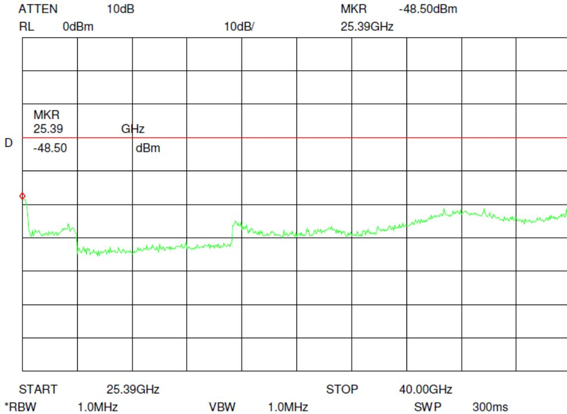
**Figure 34: 25 GHz Point to Point link spurious emissions**
