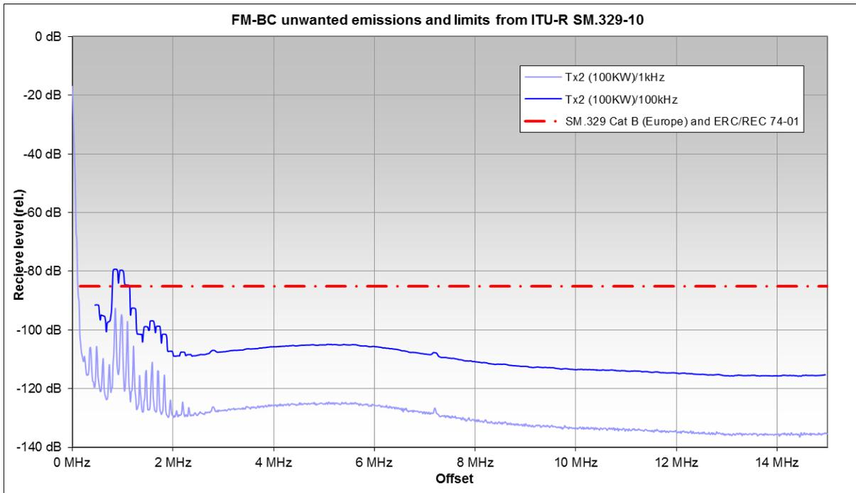
**Figure 69: Spurious emissions of a 100 kW FM broadcast transmitter (upper frequency range)**
