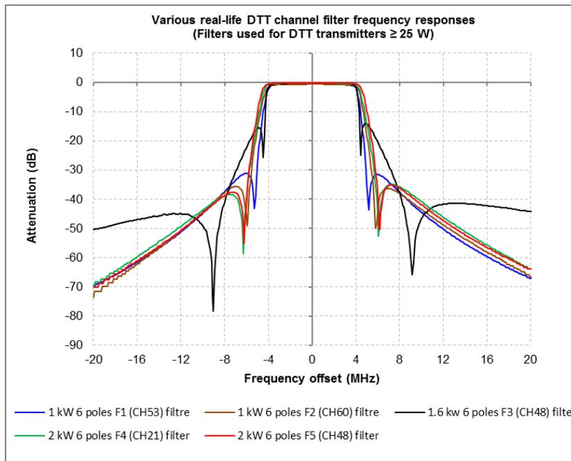
**Figure 11: Actual DTT channel filters used for high power transmitters (≥ 25 W)**
