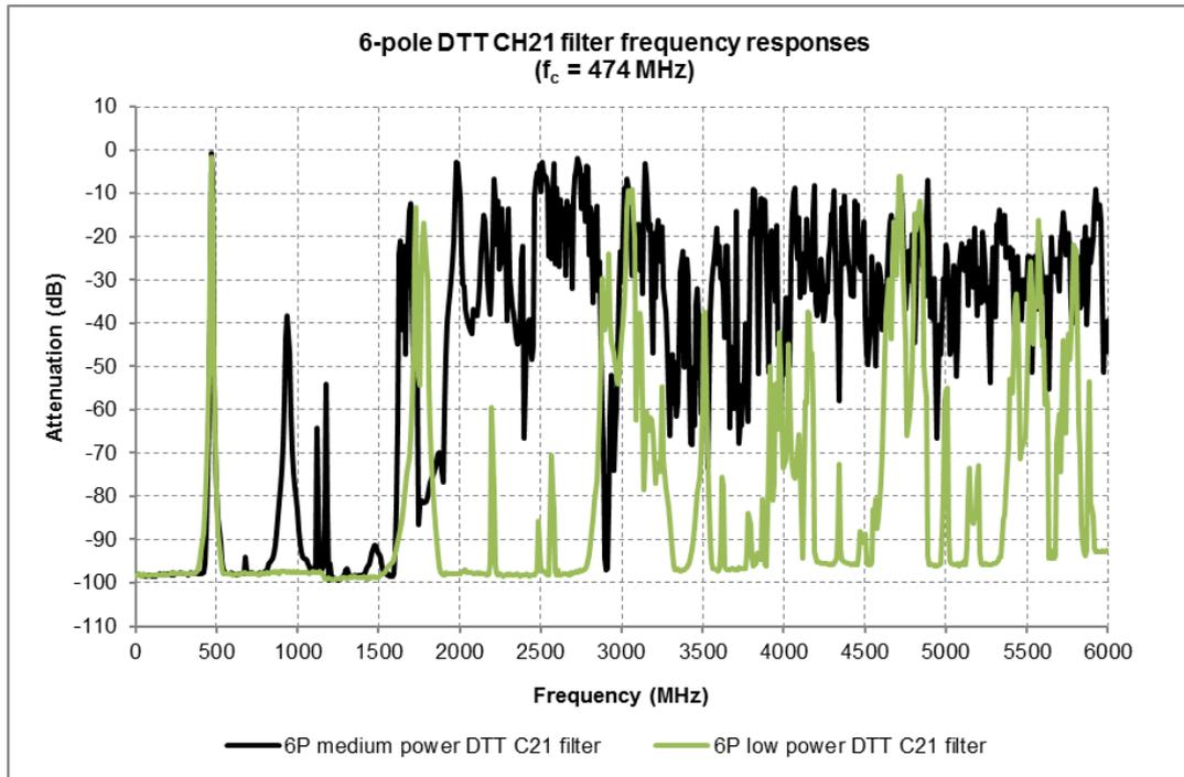
**Figure 40: Comparison of low and medium power 6-pole DTT Ch21 filter frequency responses – 0-6 GHz**
