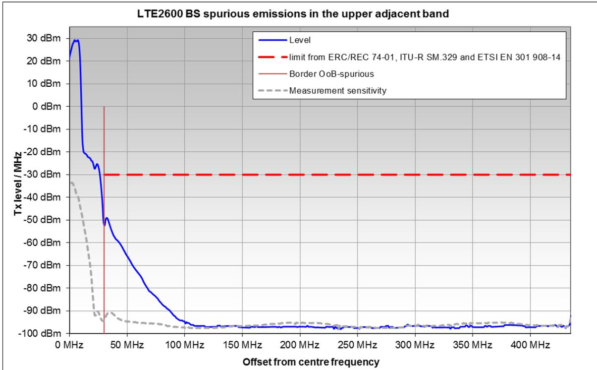
**Figure 62: LTE2600 BS spurious emissions (Bandwidth = 1 MHz)**
