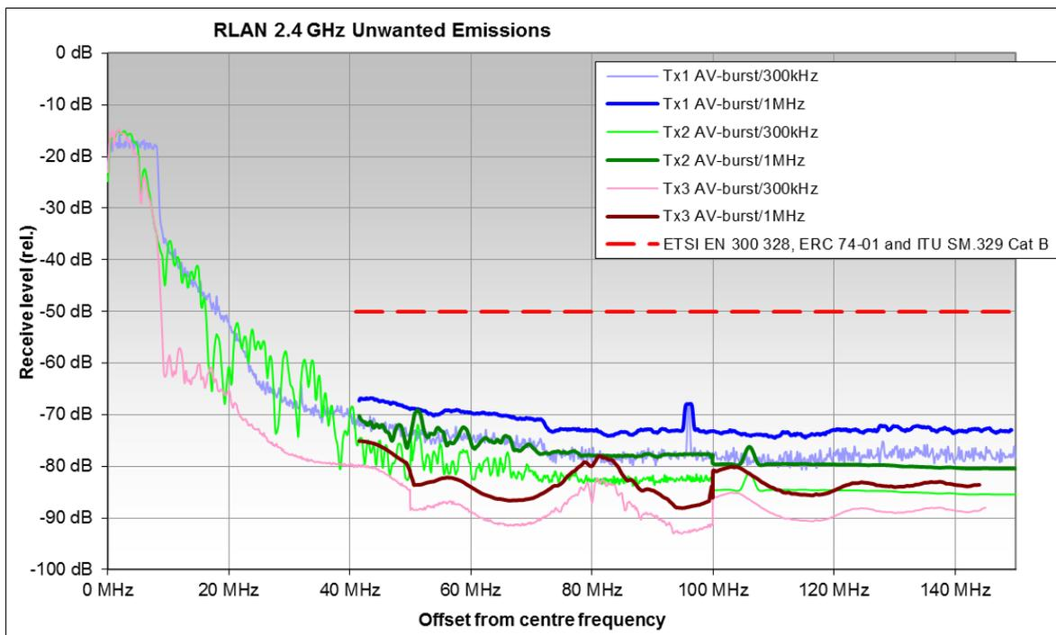
**Figure 31: RLAN spurious emissions**
