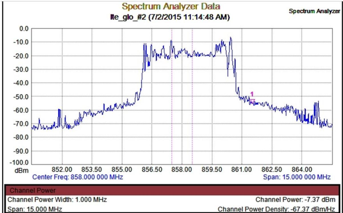
Figure 21: In-band emission from an LTE800 UE
