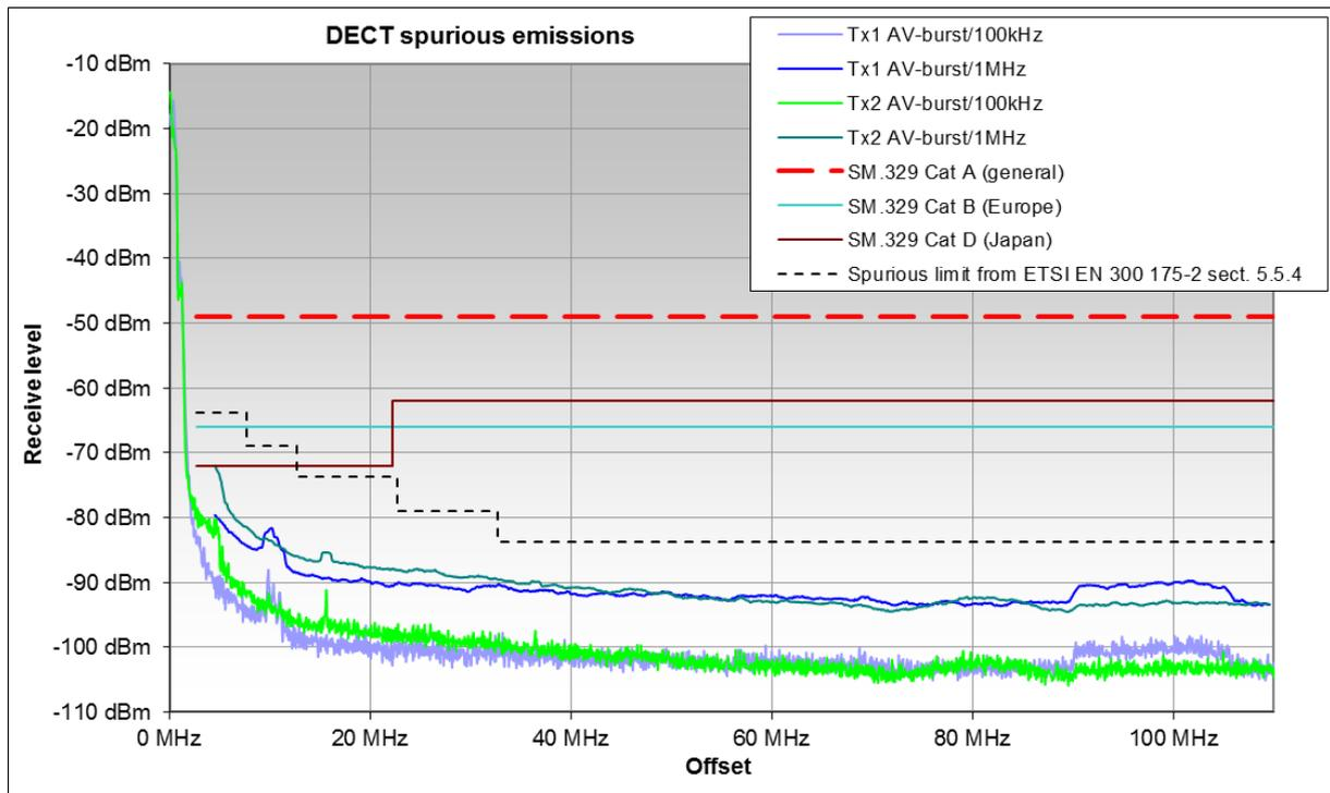
**Figure 27: DECT spurious emissions (upper frequency range)**
