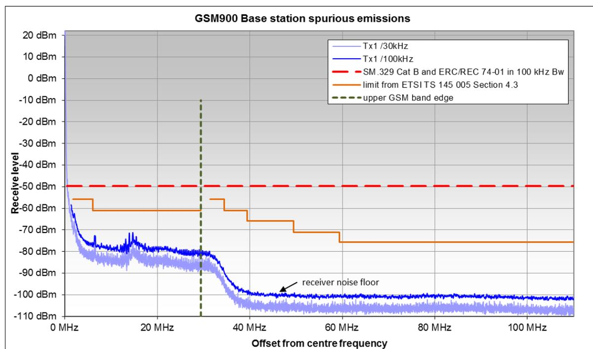
**Figure 25: GSM900 spurious emissions (upper frequency range)**
