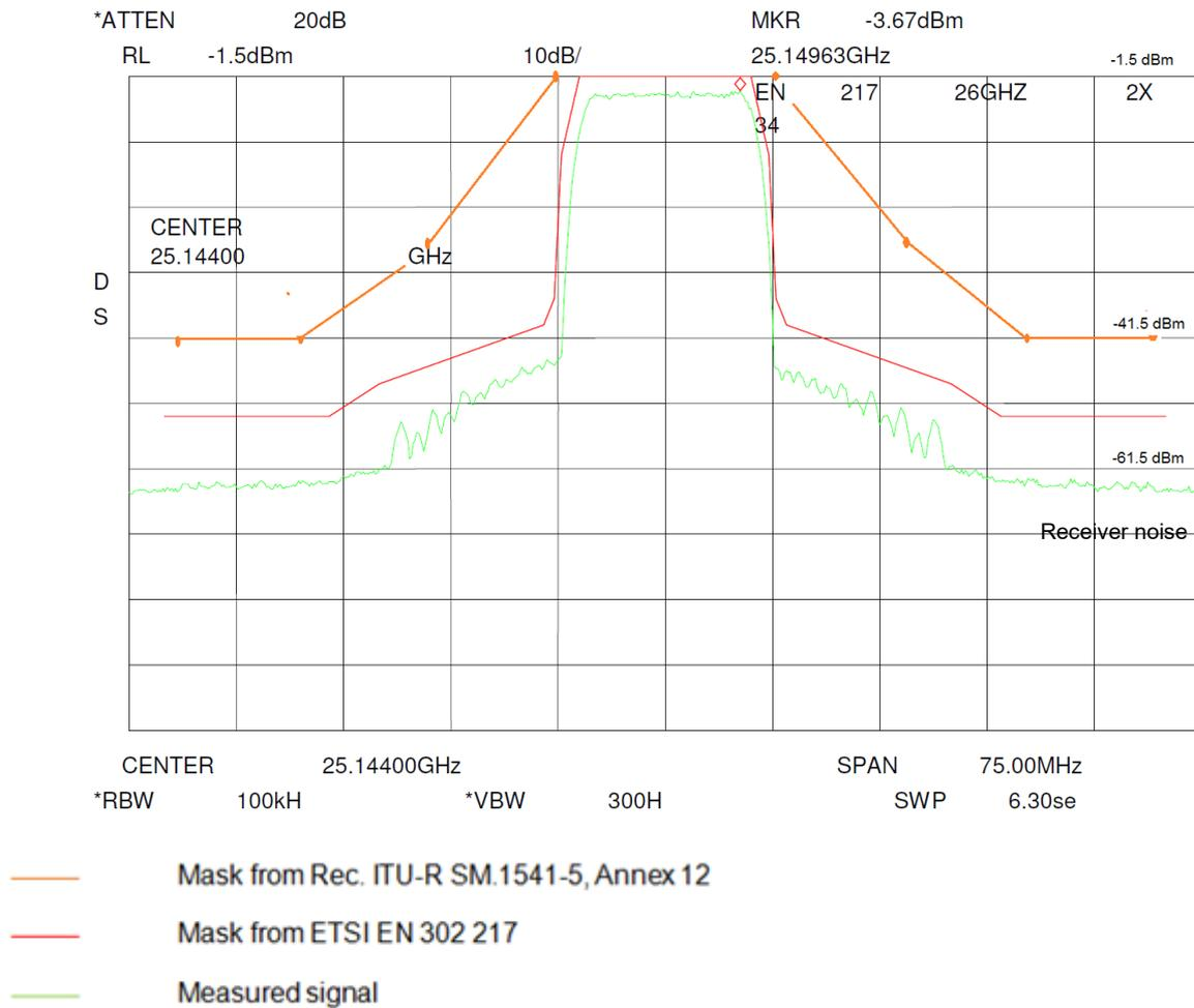
**Figure 66: 25 GHz Point to Point link unwanted emissions - Device D**
