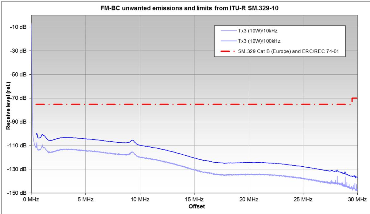
**Figure 70: Spurious emissions of a 10 W FM broadcast transmitter (upper frequency range)**
