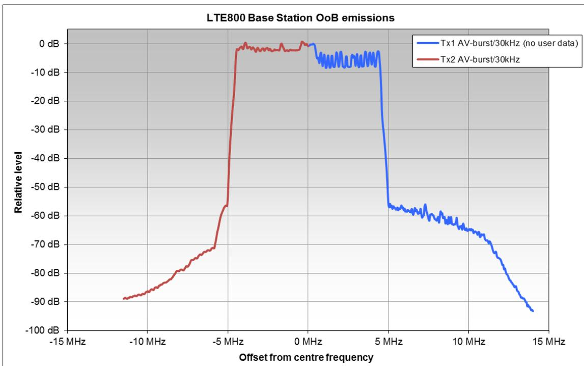
Figure 36: 'Asymmetrical' OoB spectra from an LTE800 Base Station
