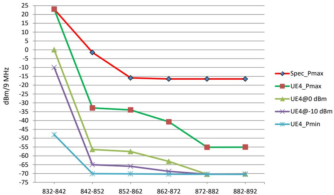
Figure 60: Measured UE#4 OoB Emissions (QPSK modulation, 12 RBs)
