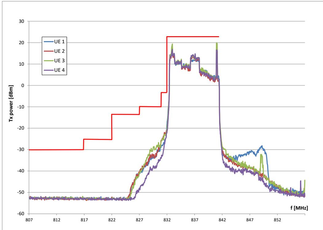
**Figure 61: Comparison of LTE UE emissions (807-857 MHz, Bandwidth = 1 MHz) vs. LTE spectrum emission mask (ETSI, 2013)**
