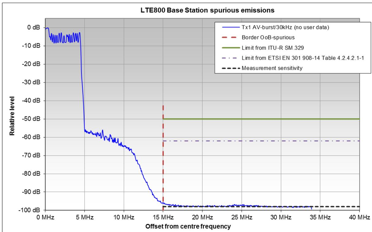
**Figure 18: Emissions from an LTE800 base station**
