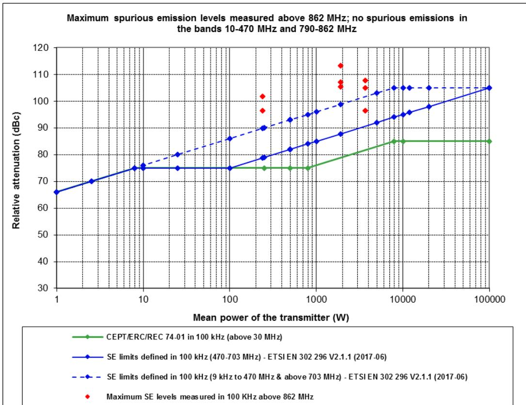
**Figure 16: High power DTT transmitters spurious emission levels**
