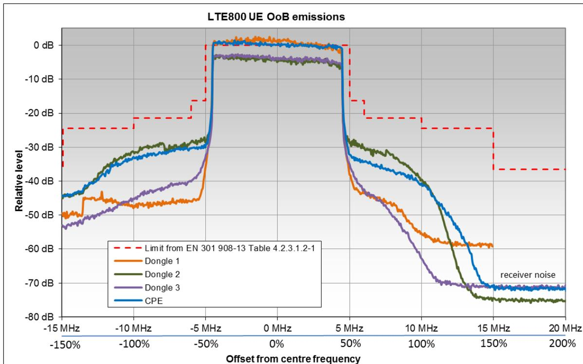
**Figure 19: OoB measurements of four LTE800 UEs**
