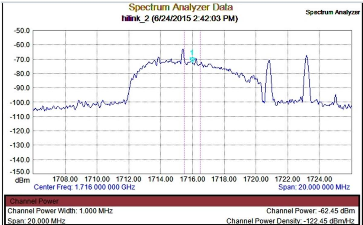
Figure 22: Emission from an LTE800 UE at the second harmonic frequency
