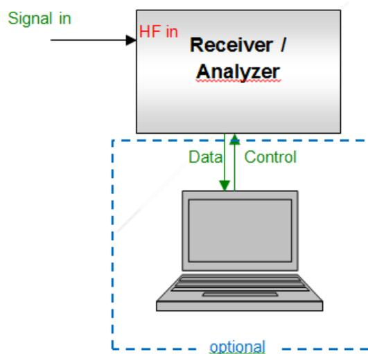
Figure 49: Principle measurement setup Type 1
