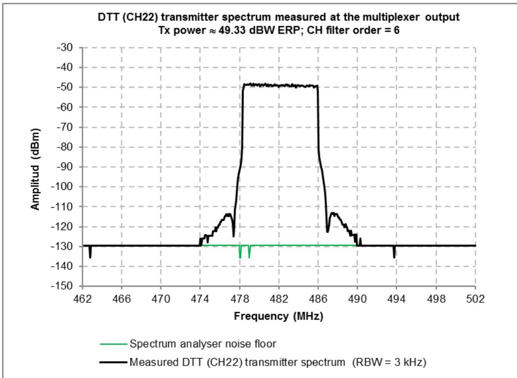
**Figure 6: Spectrum of a high power DVB-T transmitter**
