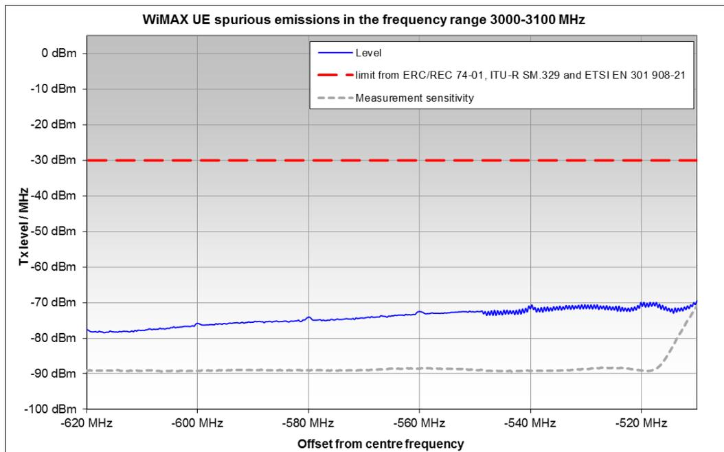
**Figure 32: UE 3.6 GHz WiMAX - Emissions in radar frequency band**
