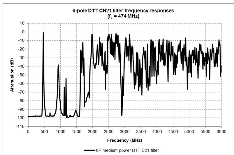
**Figure 39: 6-pole DTT Ch21 filter frequency response - 0-6 GHz**
