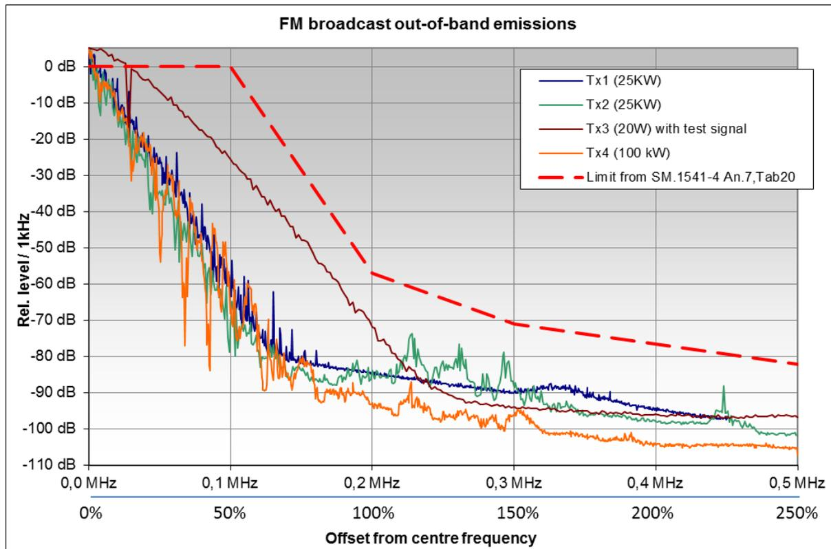
**Figure 67: OoB measurements from four different FM broadcast transmitters**
