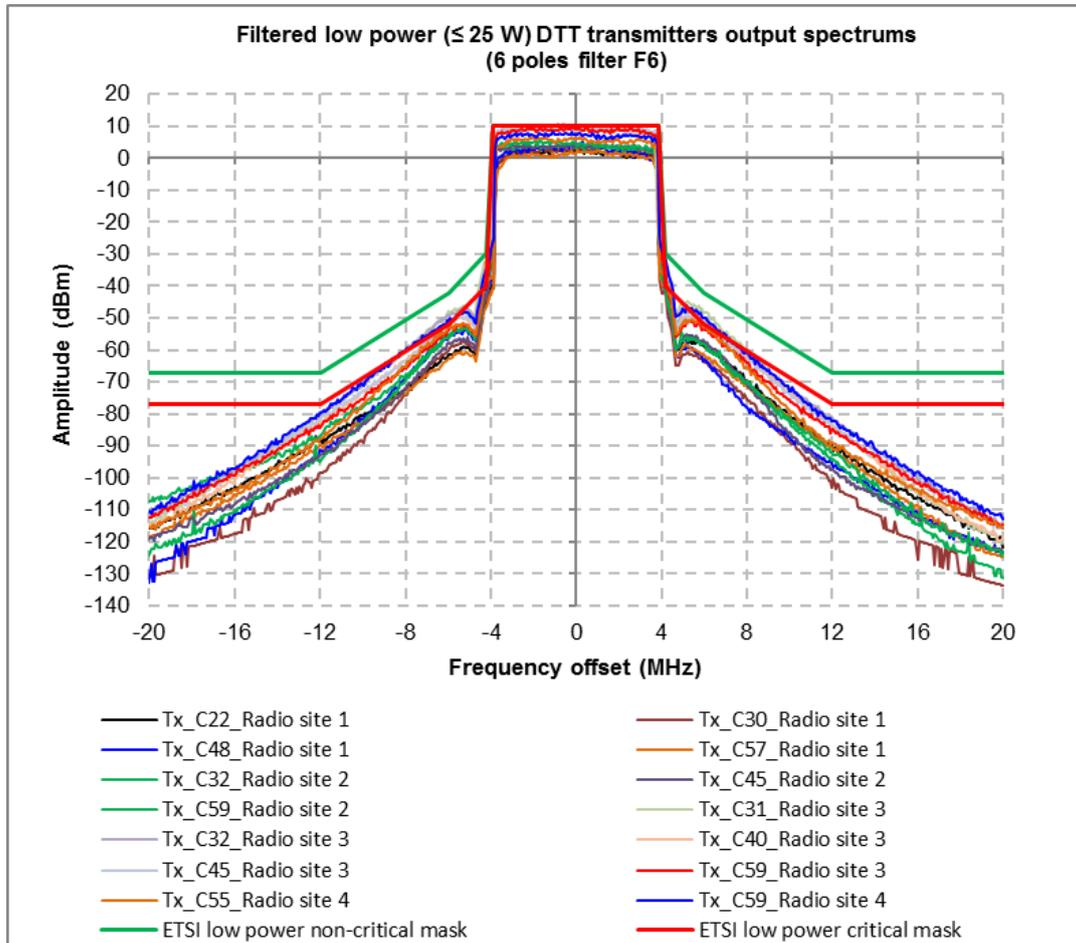
**Figure 13: Low power DTT transmitters spectrum calculated at the output of a 6-pole channel filter**
