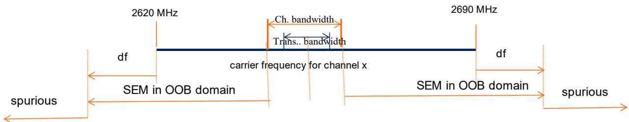
**Figure 1: Out-of-band and spurious domain for E-UTRA band 7 ( $df = 10$  MHz)**
