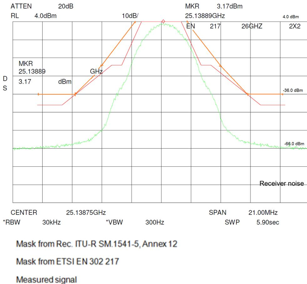
**Figure 64: 25 GHz Point to Point link unwanted emissions - Device A**
