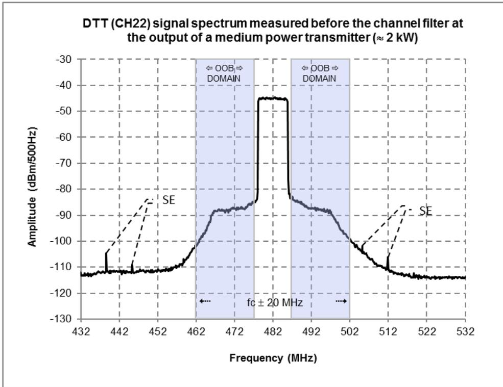
Figure 44: DTT Ch22 signal spectrum before the channel filter - 432-532 MHz
