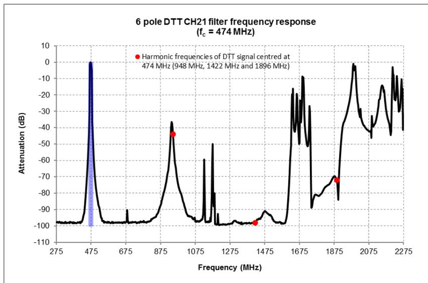
**Figure 38: 6-pole DTT Ch21 filter frequency response - 275-2275 MHz**
