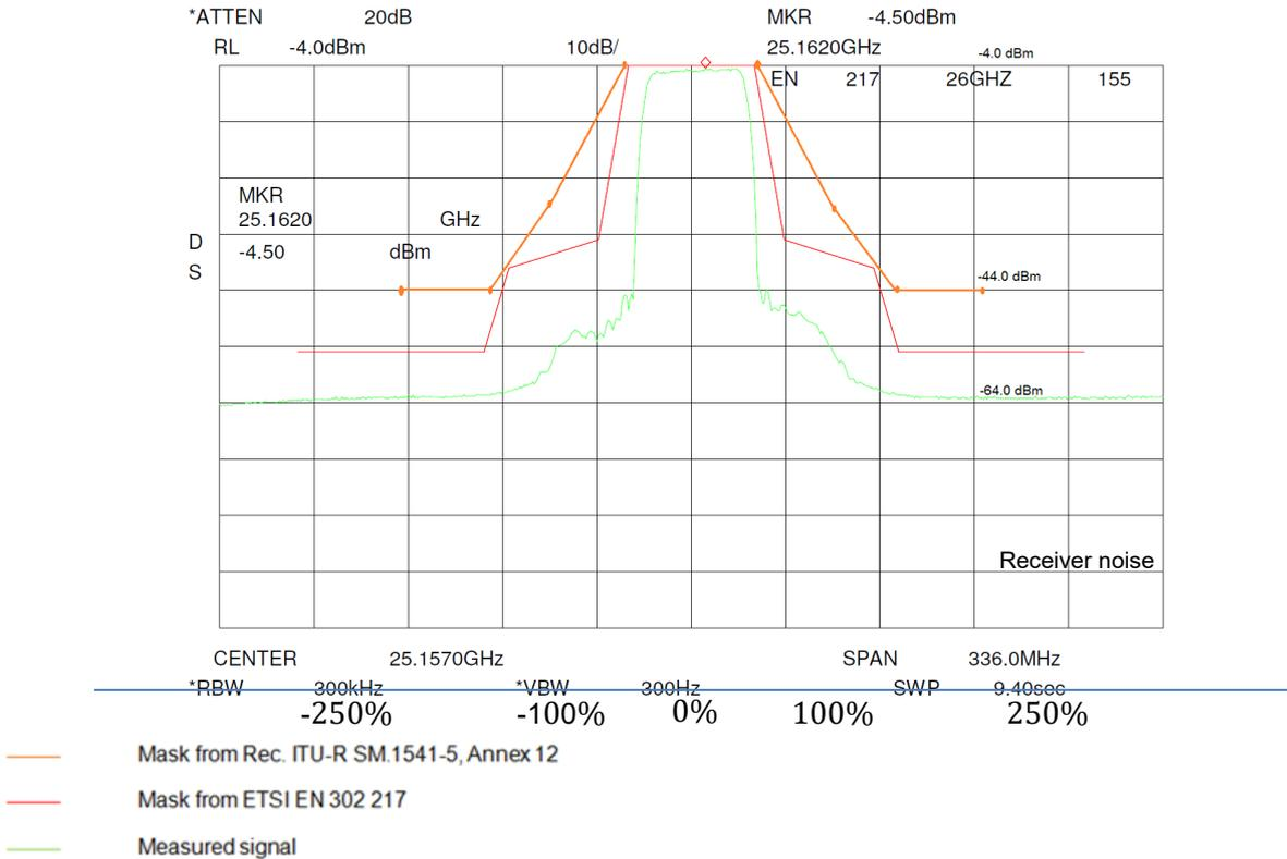
**Figure 33: 25 GHz Point-to-Point link unwanted emissions**
