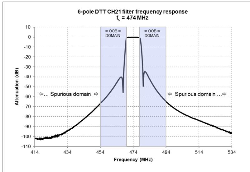
**Figure 37: 6-pole DTT Ch21 filter frequency response - 414-534 MHz**
