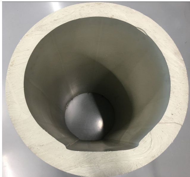
Figure 73: Cross section of a pipe where "sagging" occurred during production
