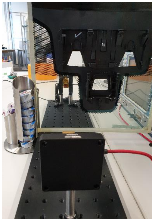
Figure 128: Photograph of the measurement position for car glass samples with camera mounting points and sun shielding
