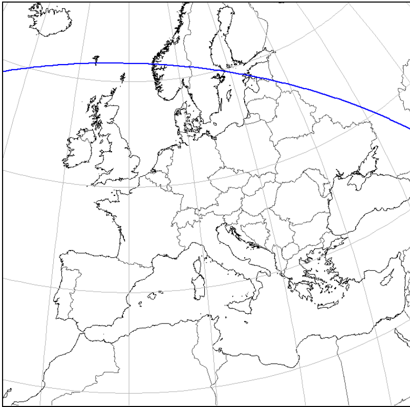
Figure 6.4.1: 20 degree elevation angle contour for Intelsat VIII Satellite @ 359°E
