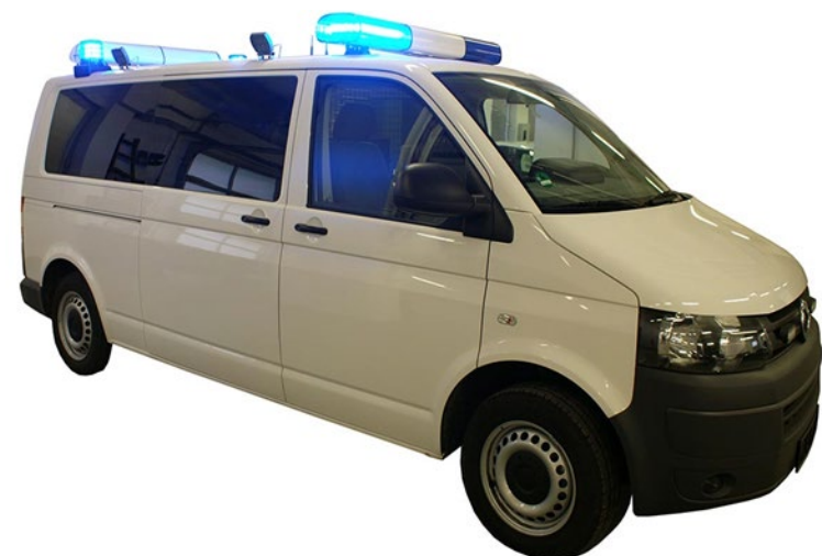
Figure 6: Typical mobile enforcement vehicle, RSU antennas are mounted on top of the roof in the back of the vehicle [5]
