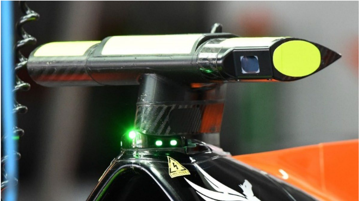
Figure 14: On-board camera, mounted above F1 car's cockpit
