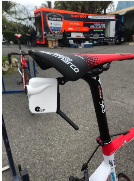
Figure 11: Rear-pointing HD camera mounted on the seat post of a Tour de France bike
