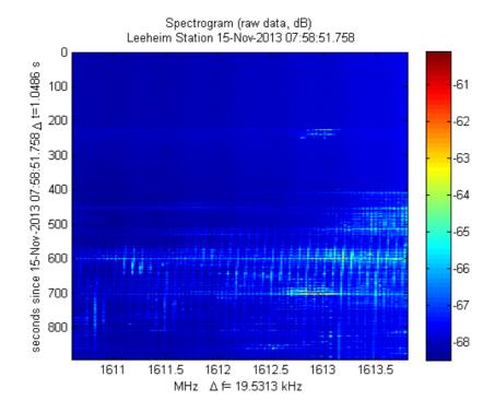
Figure 18: Spectrogram display of raw data from measurements of Iridium satellite No. 12
