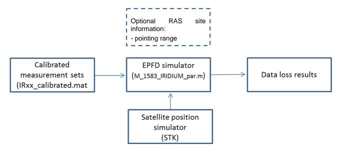
Figure 2: epfd calculations process
