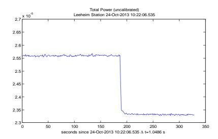
Figure 4: Total uncalibrated power from a calibration measurement, illustrating the on- and off-source positions
