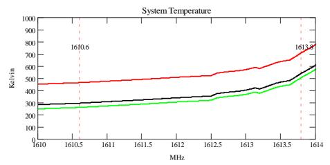
Figure 9: The green trace shows the expected system temperature at  $\phi$ =90° (zenith), the black trace at  $\phi$ =5° and the red trace at  $\phi$ =0° (horizontal). The filter loss is responsible for the majority of the system noise, only for elevations near the horizon (< 3°), one can expect a significant contribution of the ground radiation
