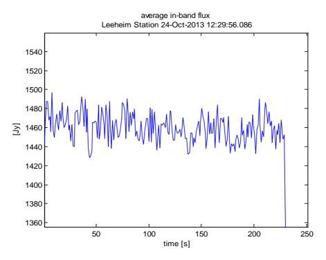
Figure 12: High resolution graph of Cas-A spectral flux density measurement
