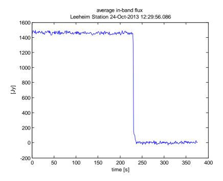
Figure 11: Calibrated total spectral flux density for a Cas-A on-off measurement
