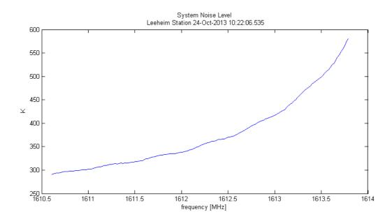
Figure 8: Measured system noise temperature as a function of frequency
