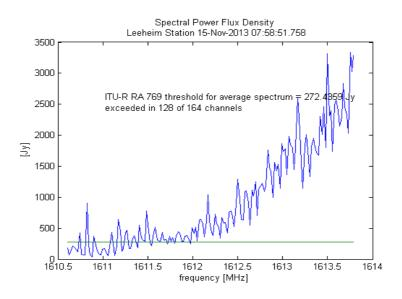
Figure 20: Time averaged spectrum. The green line is the appropriately scaled interference limit (see also examples in [5])
