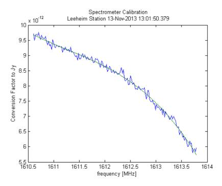
Figure 15: Calibration curve as function of frequency obtained with Cas-A
