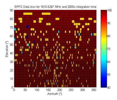
Figure 24: Result of epfd calculation at 1610.6 MHz for 2000 s integration time.
