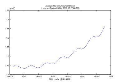
Figure 5: An interference-free band pass in a calibration measurement
