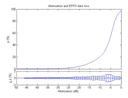
Figure 25: epfd data loss as a function of additional signal attenuation
