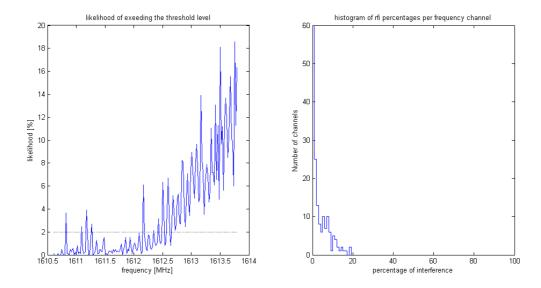
Figure 22: Graphic summary of the interference distribution. Left panel: per channel ratio of the number of 1 second samples exceeding the threshold to the total number of samples.
