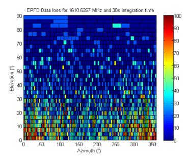
Figure 26: Result of epfd calculation for 30 s integration time. Percentages are colour coded
