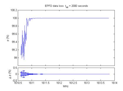
Figure 28: percentage of data loss in the band 1610.60-1613.80 MHz for 2000s of integration time
