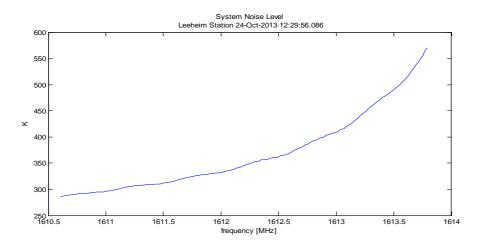
Figure 13: System noise temperature (K) as calibrated on Cyg-A
