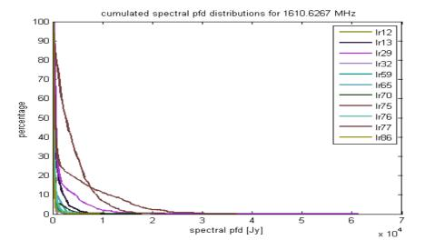
Figure 23: Cumulated spectral power flux density distributions for different Iridium satellites at 1610.6 MHz
