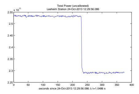
Figure 10: Total uncalibrated in-band power for Cas-A measurement in spectrometer units
