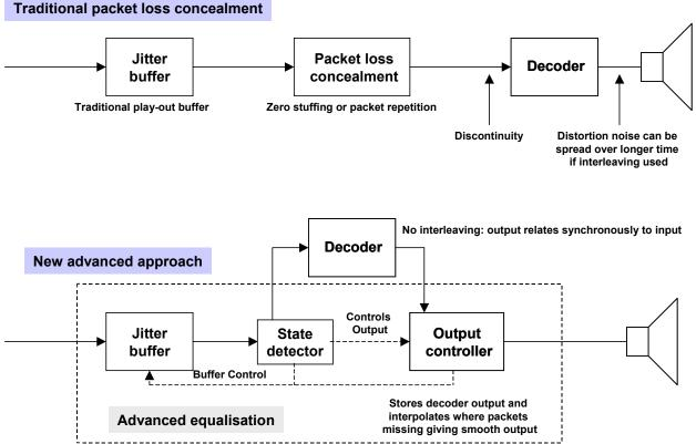
Figure 9: Simple block diagram depicting how an advanced algorithm can interacts with the speech decoder and the jitter buffer
