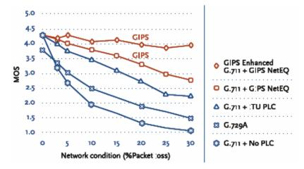
Figure 11: Narrowband performance improvements in presence of packet loss (Source: Lockheed Martin - COMSAT)
