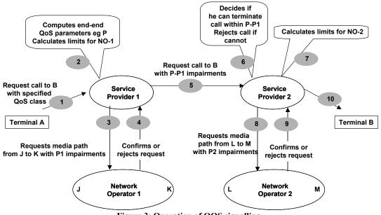
Figure 3: Operation of QOS signalling
