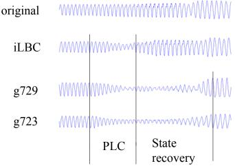
Figure 7: Recovery from packet loss
