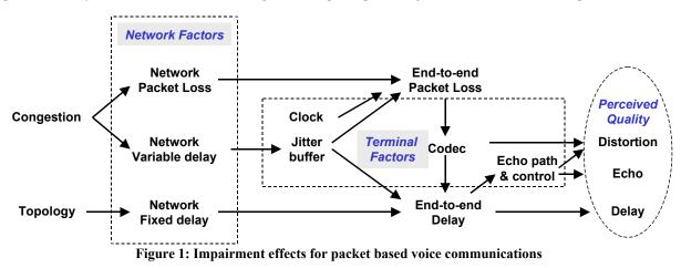
The figure distinguishes between the effects that occur in the network and the mechanisms in the terminals that are affected and that can be used to correct for the effects in the network. The network fixed delay is sometimes called the transmission or propagation delay.
