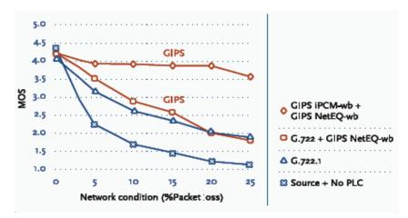
Figure 12: Wideband performance improvements in presence of packet loss (Source: Lockheed Martin - COMSAT)
