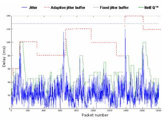
**Figure 10: Delay performance for different playout buffers on a system with 20 ms packets.** (Note that the constant system delays of about 80ms have been removed from all curves.)
