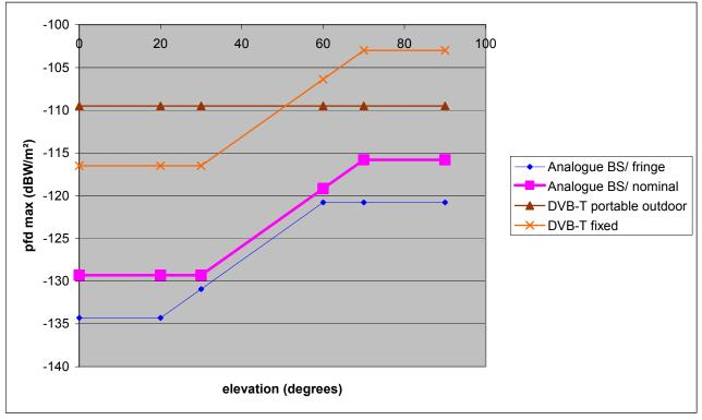
Figure 1: Maximum interfering pfd levels at BS receivers
