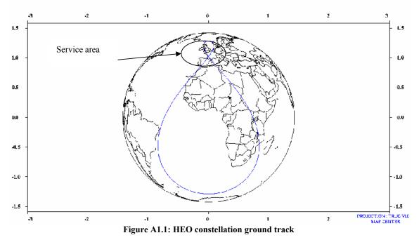
Figure A1.1 illustrates the satellite's ground track on the Earth's surface.
