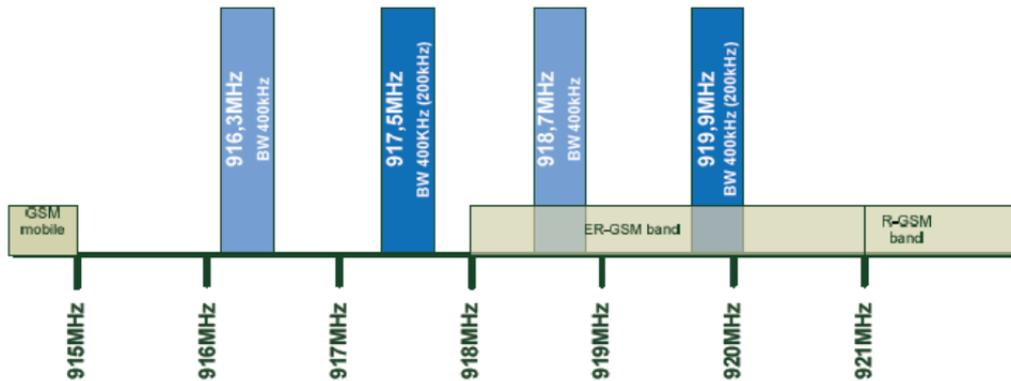
**Figure 3: Tentative band plan for 915-921 MHz, based on amended TR 102 649-2 [2] proposal**
