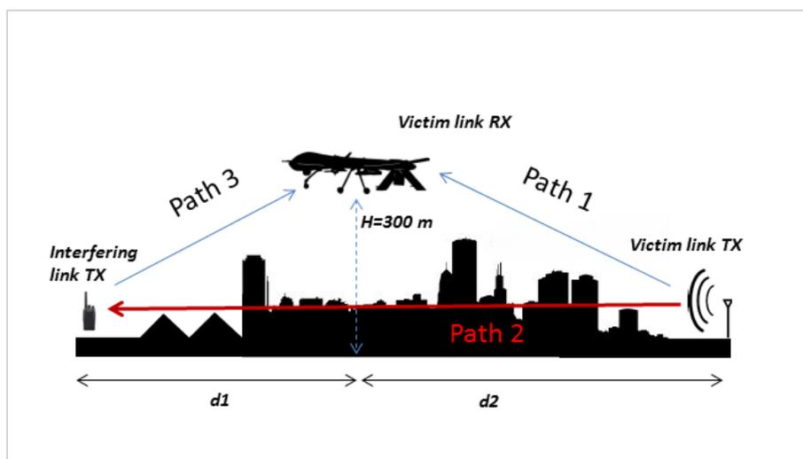
**Figure 44: Considered DAA sensing configuration for UAS scenarios**
