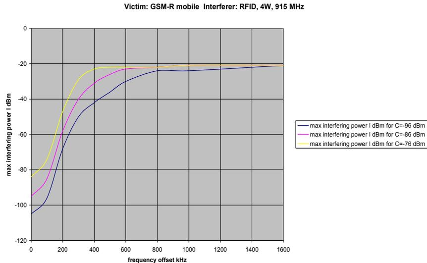
**Figure 55: Main results of ETSI TR 101 537: max acceptable interference power at ER-GSM receiver**
