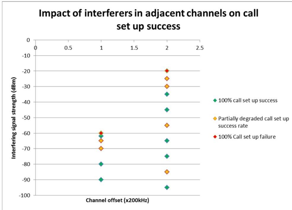
**Figure 53: Detailed measurements of the impact of a 100% DC interferer in adjacent channels on call set up success (wanted signal -91dBm)**
