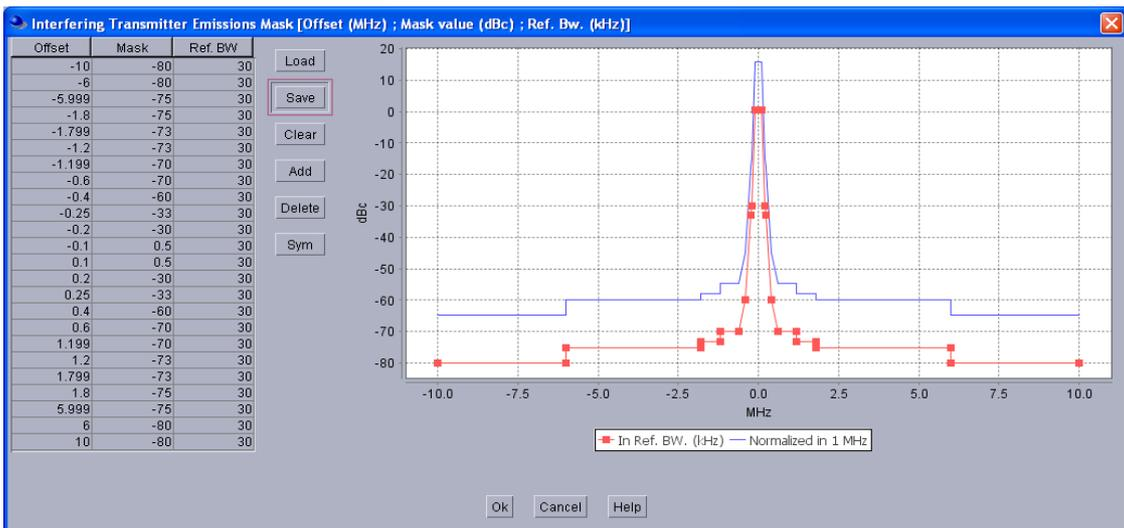
Figure 18: Unwanted emissions mask of GSM-R BTS [22]
