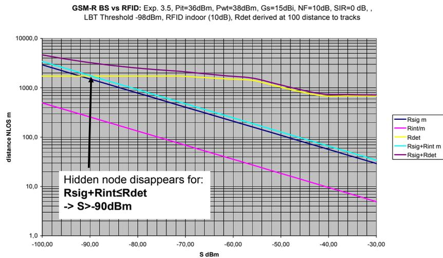
**Figure 65: Calculated area sizes for indoor RFID case**
