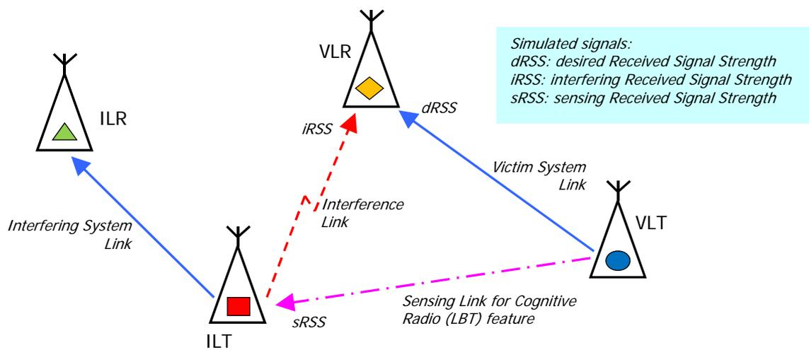
**Figure 39: Modernised representation of SEAMCAT scenario elements**
