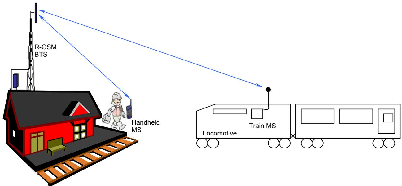
**Figure 14: Different types of stations/users in GSM-R**
