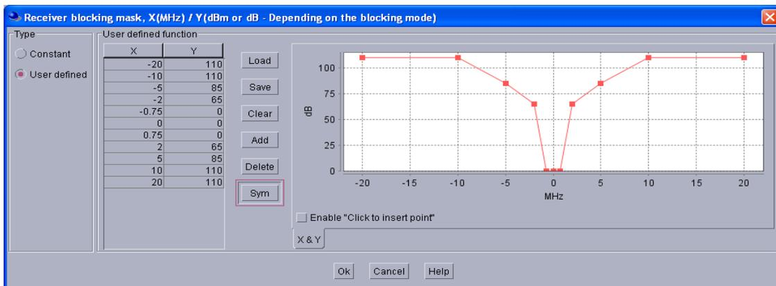
Figure 25: Receiver blocking function of TRR (ref. STANAG-4212 [18])
