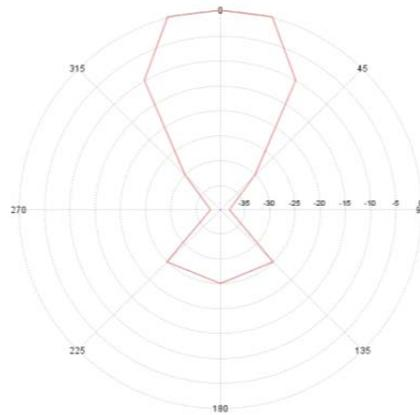
**Figure 69: Horizontal antenna pattern of RFID Type 2 antenna**
