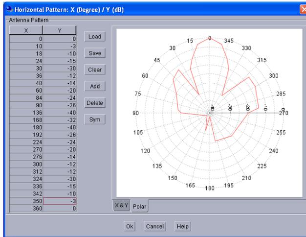
Figure 23: Radiation pattern of TRR antenna [18]
