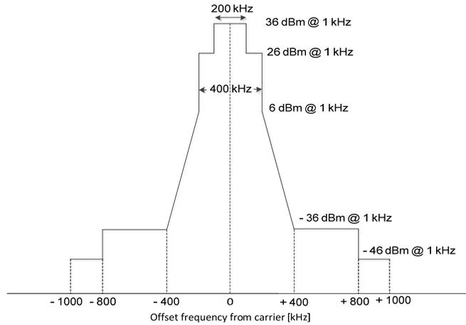
**Figure 31: Spectrum emissions mask of RFID interrogator's transmitter**
