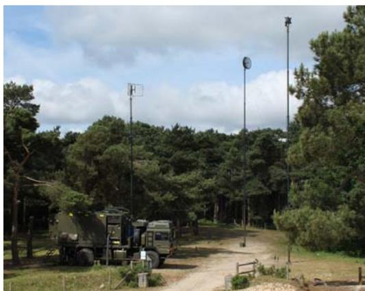
**Figure 42: Practical example of TRR antennas mounted above clutter**
