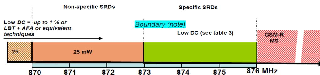
NOTE: It is expected that the boundary between non-specific and specific SRDs will lie somewhere between 873 MHz and 874 MHz. The exact frequency will be determined following the compatibility study when the impact of GSM-R on the upper part of the band has been quantified. It should be noted that specific SRDs have a minimum requirement for 2 MHz of usable spectrum.
