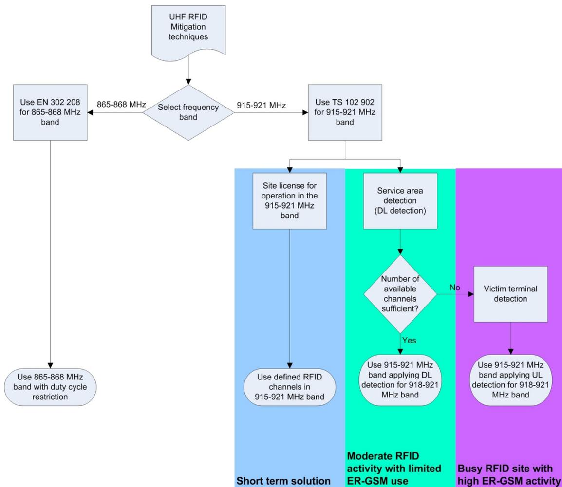
**Figure 60: Overall coexistence strategy between ER-GSM and RFID**
