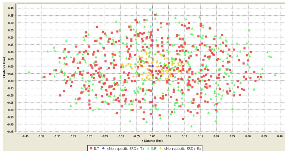
**Figure 12: Example of SEAMCAT simulation window: Intra-SRD co-existence scenario**
