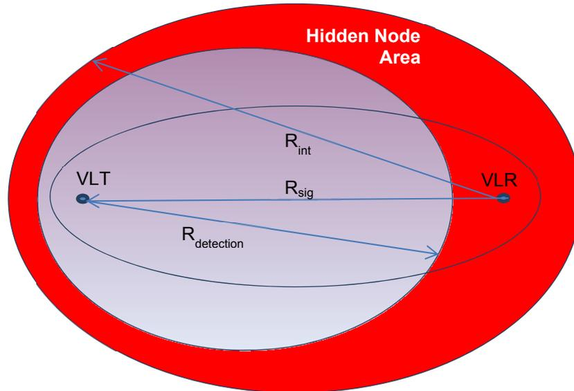
**Figure 41: Illustration of DAA sensing deficiency (Hidden Node)**
