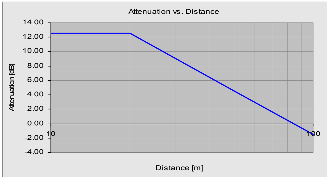
Figure A3.7. Attenuation versus Distance required due to wide band noise
