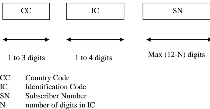
**Figure 3: International Public Telecommunication Number Structure for International Networks**
