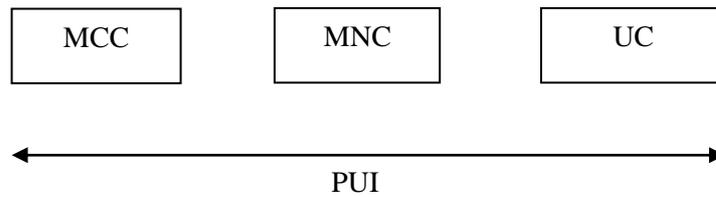
**Figure 2: Structure of PUI**
