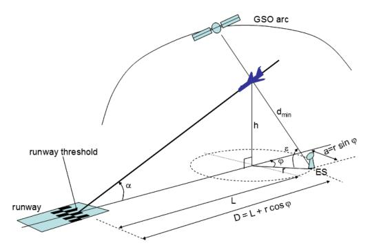
Figure 1: Scenario when aircraft crosses the main beam of an earth station
