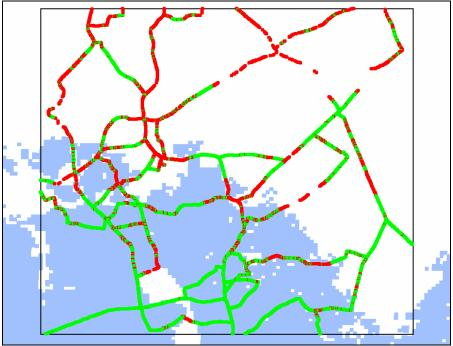
Figure 8: Sample measurement route inside a reference area. Green indicates RSCP better than -114 dBm (network login possible)
