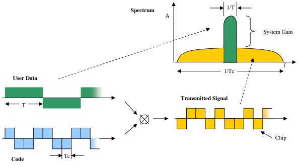
Figure 1: Principle of spectrum spreading
