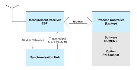
Figure 9: Hardware setup used in Germany
