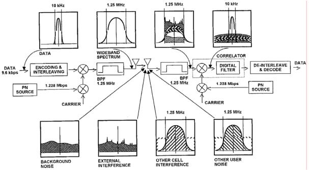
Figure 2: Used and interference spectra at different stages of the transmission process (example from IS-95)
