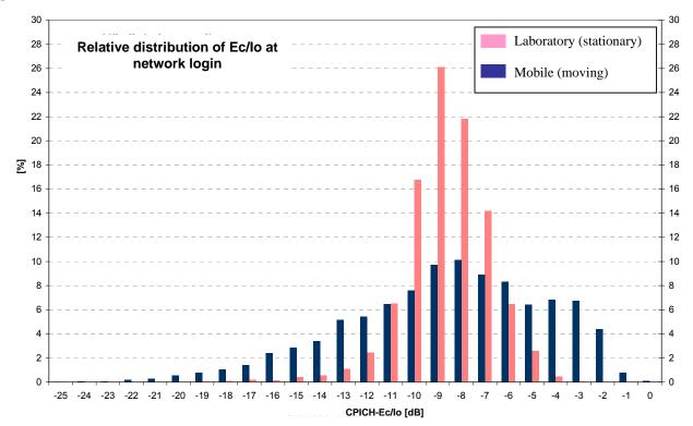
Figure 4: Ec / Io values at network login
