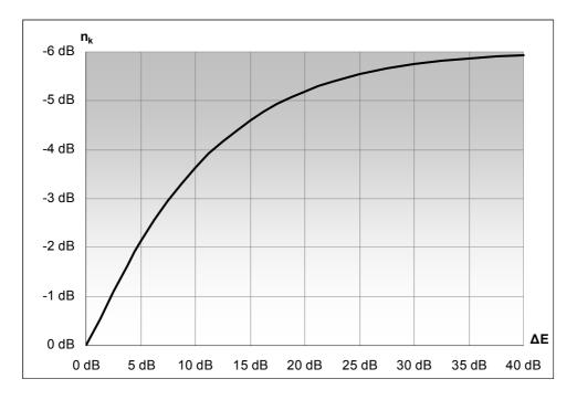
Figure 2: Correction curve for n<sub>k</sub>
