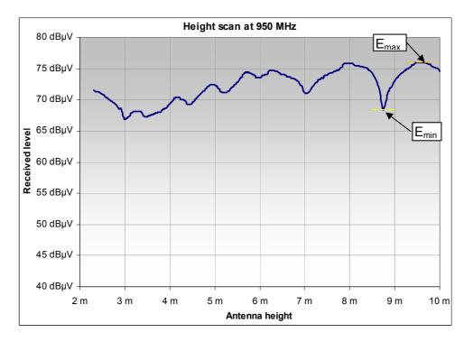
Figure 1: Example of the dependency of the measured field strength on measurement antenna height
